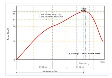
Fig 2. Infrared soldering profile
