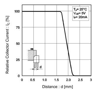
Fig.2 Relative Output Current vs.Distance (II)
