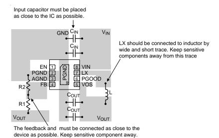
Figure 3. PCB Layout Guide
