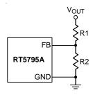
Figure 1. Setting the Output Voltage
