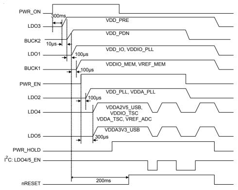
Figure 7. RT9941 POWER ON/OFF Timing Diagram
