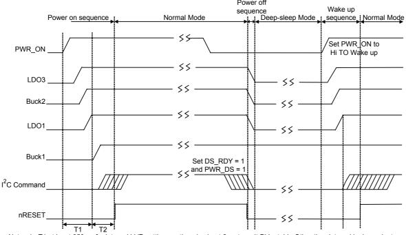
Notes 1: T1 at least 650µs for internal LVR setting up time, is about 2ms to wait PLL stable Other time interval is dependent on power stable. Notes 2: After wake up sequence from Deep-sleep Mode, the power on sequence to Normal Mode is similar to when powering on initially.
