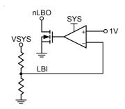
Figure 22. LBI and nLBO Application Circuit
