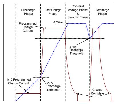
Figure 14. Typical Charge Profile
