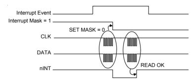
Figure 10. Interrupt with Mask
