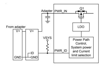
Figure 18. RT9941 Powered by AC Adapter
