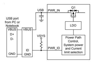
Figure 19. RT9941 Powered by USB Port
