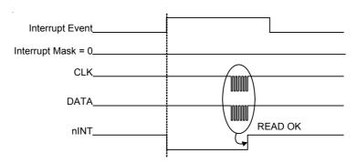
Figure 9. Interrupt without Mask
