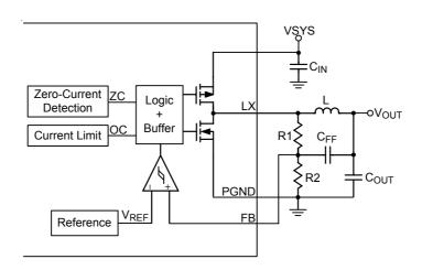
Figure 12. Step-down Converter Block Diagram
