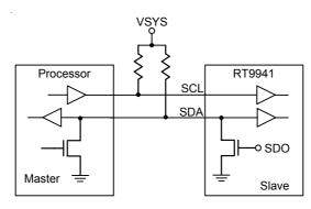
Figure 2. I<sup>2</sup>C Function Block in the RT9941
