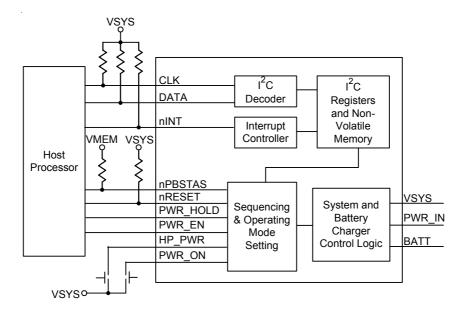
Figure 6. Power and Interface Module
