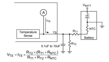
Figure 21. Connection of Battery Temperature Monitor
