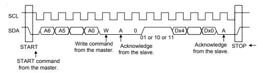
Figure 1. I<sup>2</sup>C Transmission Flow in the RT9941
