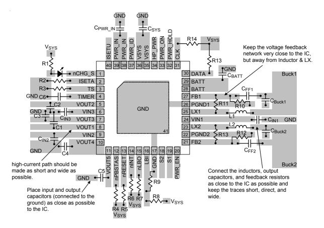
Figure 25. PCB Layout Guide
