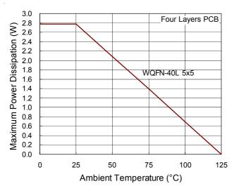
Figure 24. Derating Curves for RT9941 Packages
