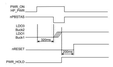
Figure 11. PWR\_ON & HP\_PWR & nPBSTAS Timing Diagram
