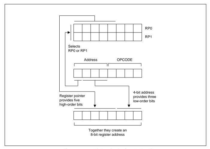
Figure 2-12 4-bit Working Register Addressing
