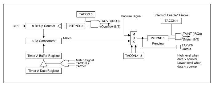
Figure 11-3 Simplified Timer A Function Diagram: PWM Mode
