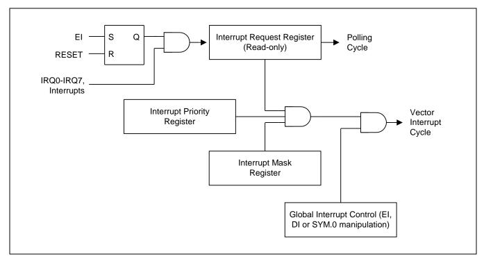
Figure 5-4 Interrupt Function Diagram
