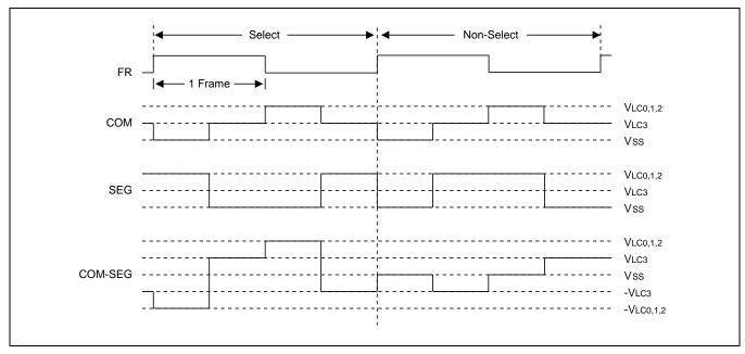
Figure 15-9 Select/No-Select Signal in 1/2 Duty, 1/2 Bias Display Mode
