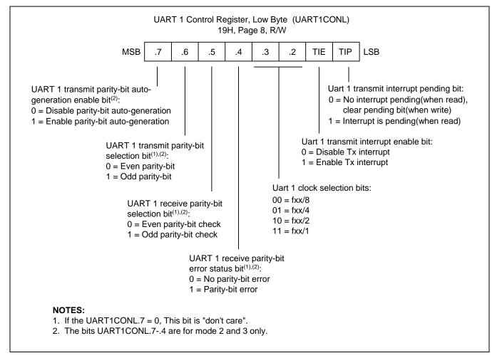
Figure 19-2 UART 1 Low Byte Control Register (UART1CONL)
