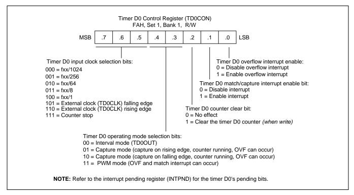
Figure 13-1 Timer D0 Control Register (TD0CON)
