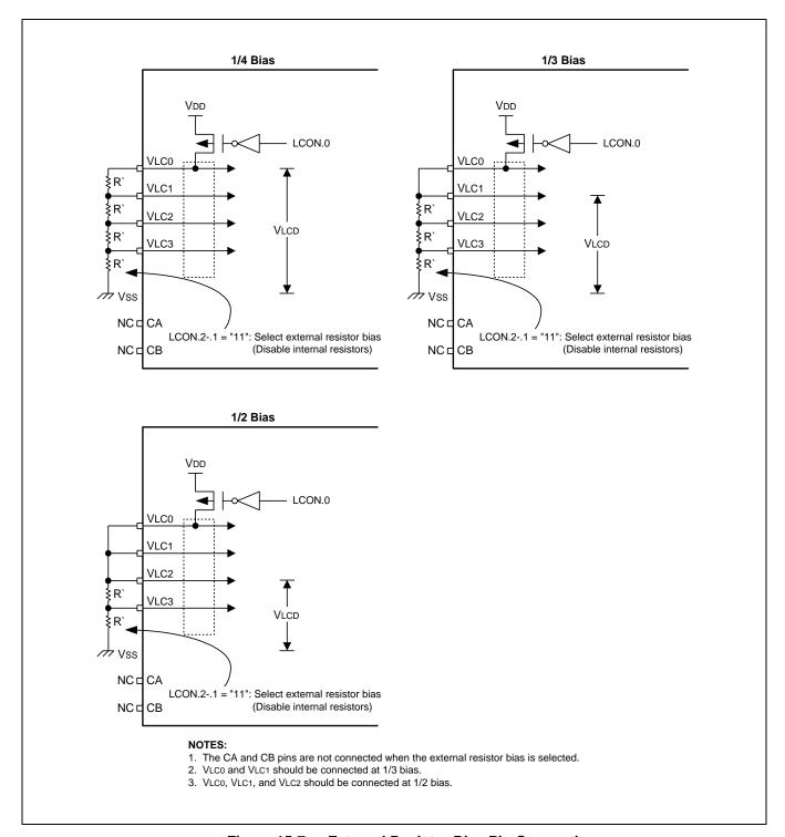
Figure 15-7 External Resistor Bias Pin Connection
