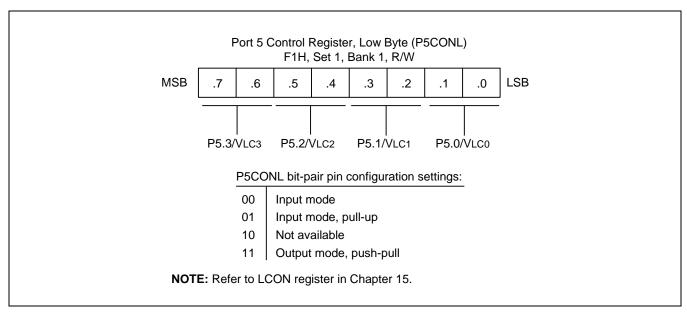
Figure 9-24 Port 5 Low-Byte Control Register (P5CONL)
