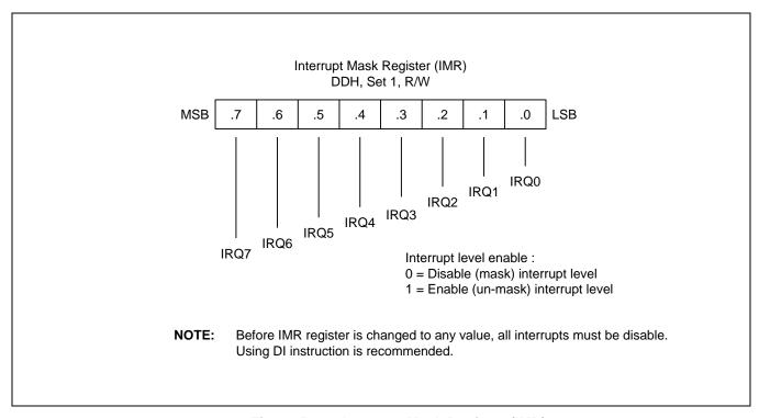
Figure 5-6 Interrupt Mask Register (IMR)
