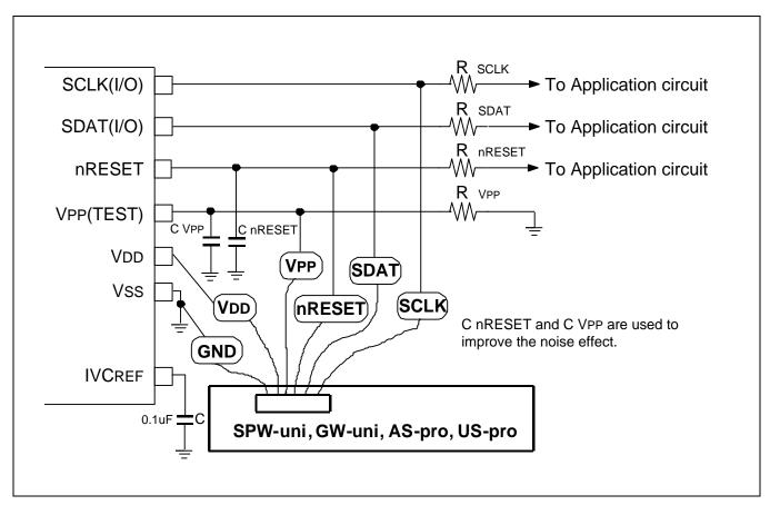
Figure 24-5 PCB Design Guide for on Board Programming
