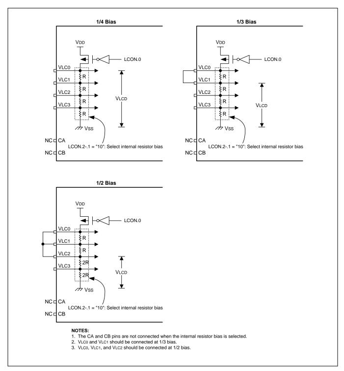
Figure 15-6 Internal Resistor Bias Pin Connection
