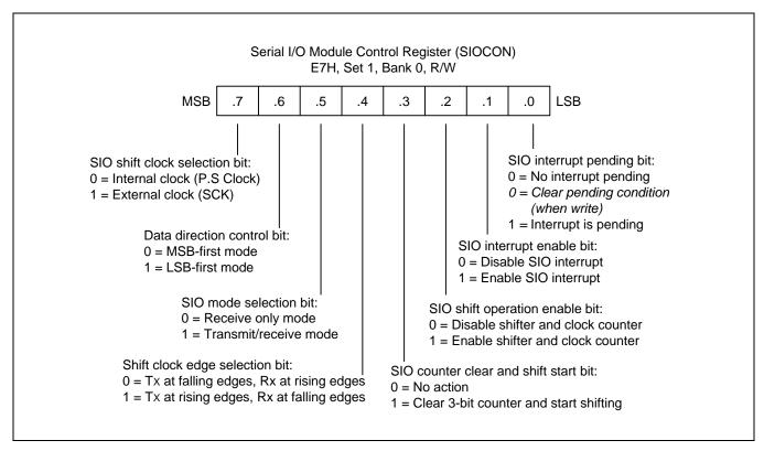
Figure 17-1 Serial I/O Module Control Registers (SIOCON)
