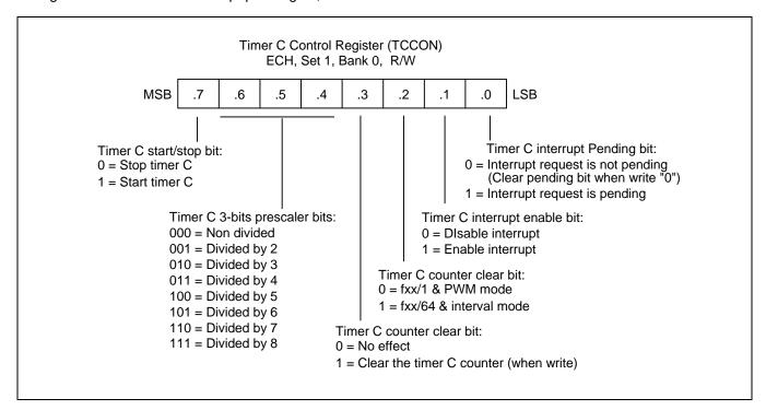
Figure 12-1 Timer C Control Register (TCCON)
