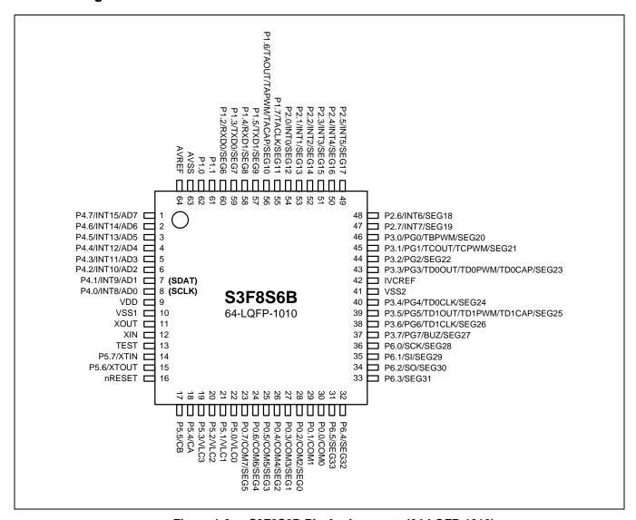
Figure 1-2 S3F8S6B Pin Assignments (64-LQFP-1010)
