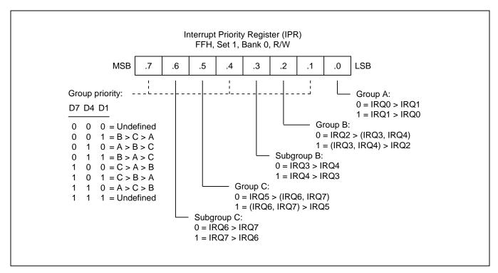
Figure 5-8 Interrupt Priority Register (IPR)
