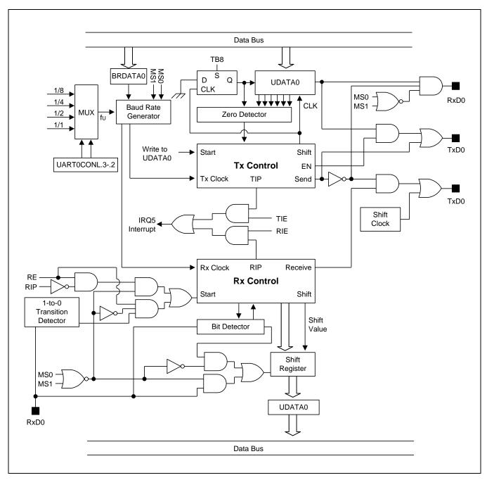
Figure 18-5 UART 0 Functional Block Diagram
