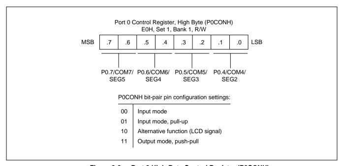
Figure 9-2 Port 0 High-Byte Control Register (P0CONH)
