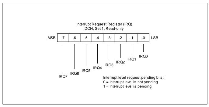
Figure 5-9 Interrupt Request Register (IRQ)
