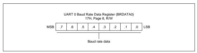
Figure 18-4 UART 0 Baud Rate Data Register (BRDATA0)
