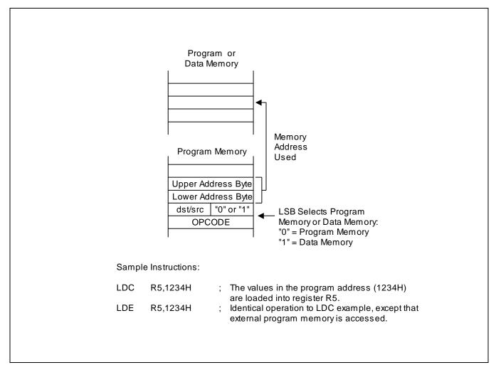
Figure 3-10 Direct Addressing for Load Instructions
