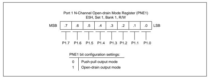
Figure 9-7 Port 1 N-Channel Open-drain Mode Register (PNE1)
