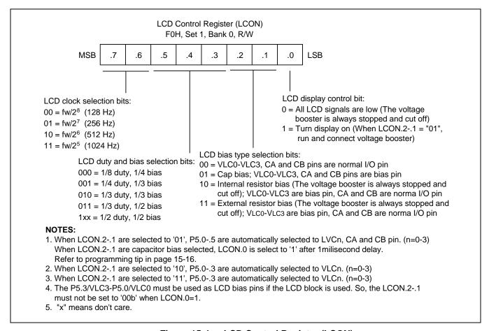
Figure 15-4 LCD Control Register (LCON)
