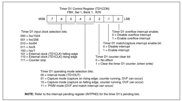
Figure 13-6 Timer D1 Control Register (TD1CON)
