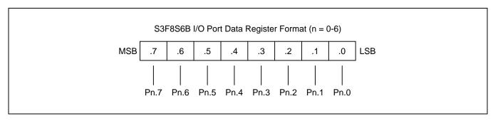
Figure 9-1 S3F8S6B I/O Port Data Register Format
