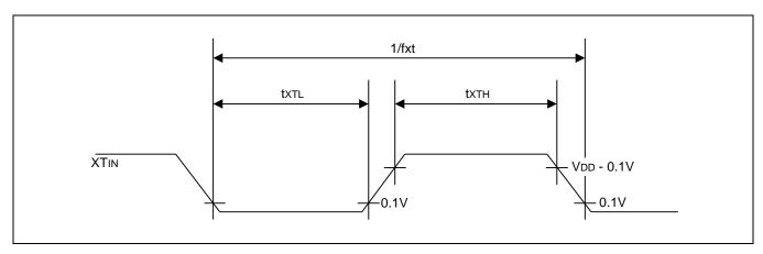
Figure 22-10 Clock Timing Measurement at XT<sub>IN</sub>
