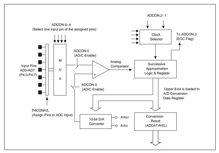
Figure 16-3 A/D Converter Functional Block Diagram
