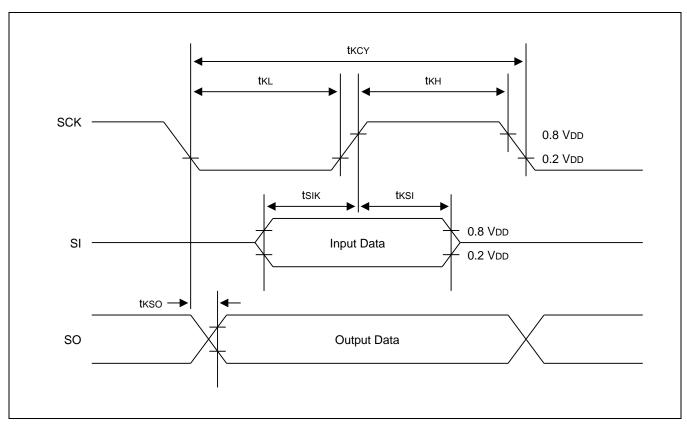
Figure 22-6 Serial Data Transfer Timing
