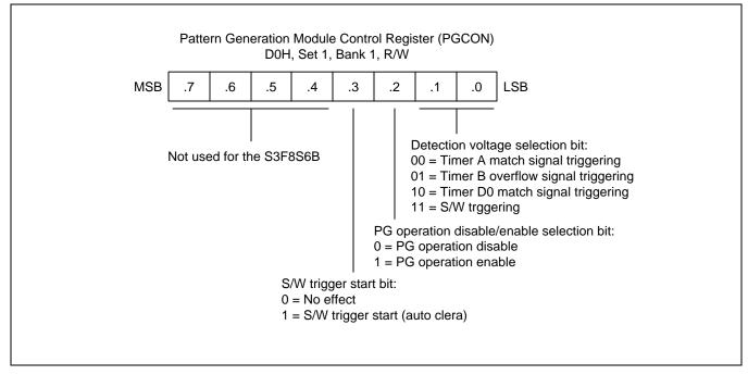
Figure 20-2 Pattern Generation Control Register (PGCON)
