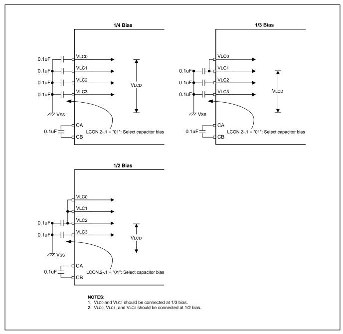
Figure 15-8 Capacitor Bias Pin Connection
