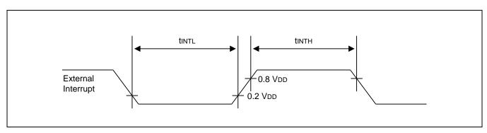
Figure 22-1 Input Timing for External Interrupts
