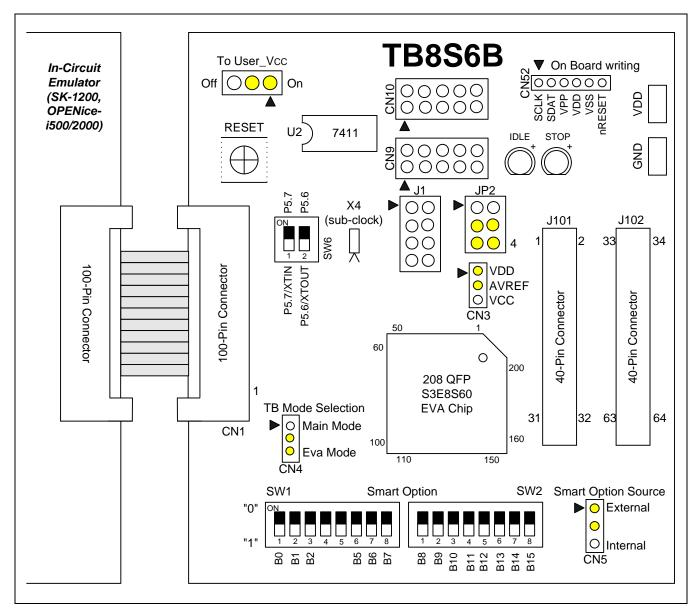
Figure 25-2 TB8S6B Target Board Configuration
