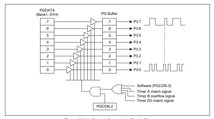
Figure 20-3 Pattern Generation Circuit Diagram
