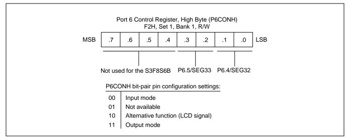
Figure 9-25 Port 6 High-Byte Control Register (P6CONH)
