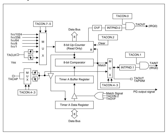
Figure 11-5 Timer A Functional Block Diagram
