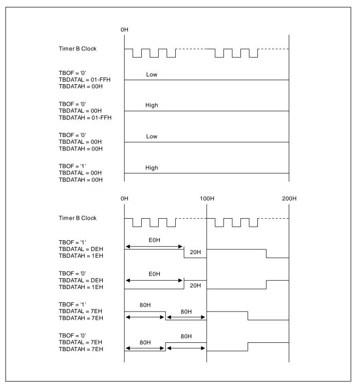
Figure 11-8 Timer B Output Flip-Flop Waveforms in Repeat Mode
