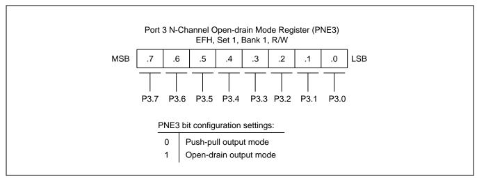
Figure 9-17 Port 3 N-Channel Open-Drain Mode Register (PNE3)
