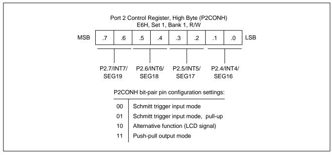
Figure 9-8 Port 2 High-Byte Control Register (P2CONH)
