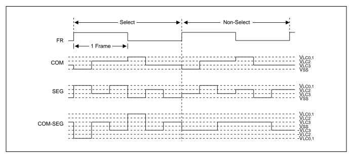
Figure 15-10 Select/No-Select Signal in 1/3 Duty, 1/3 Bias Display Mode
