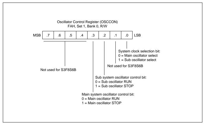
Figure 7-8 Oscillator Control Register (OSCCON)
