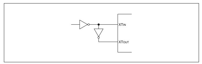
Figure 7-5 External Oscillator (fxt)
