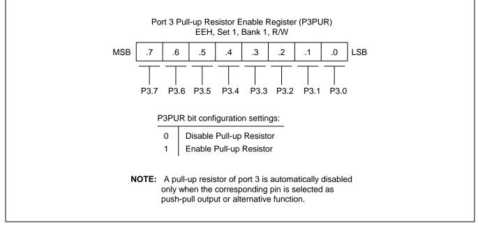
Figure 9-16 Port 3 Pull-Up Resistor Enable Register (P3PUR)
