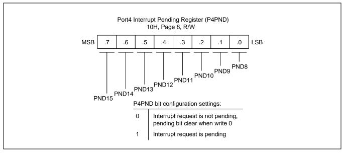
Figure 9-22 Port 4 Interrupt Pending Register (P4PND)
