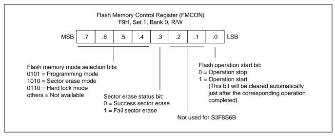
Figure 21-1 Flash Memory Control Register (FMCON)
