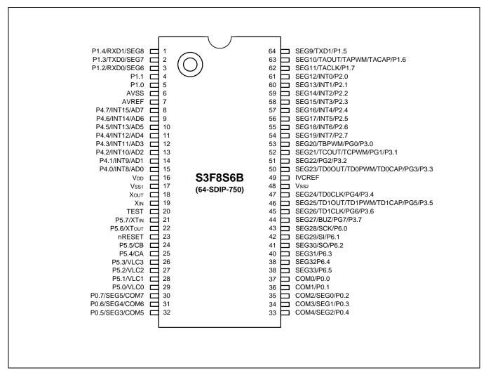
Figure 1-4 S3F8S6B Pin Assignments (64-SDIP-750)
