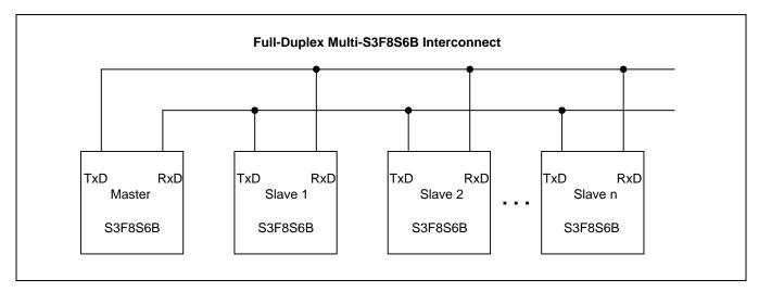
Figure 18-10 Connection Example for Multiprocessor Serial Data Communications
