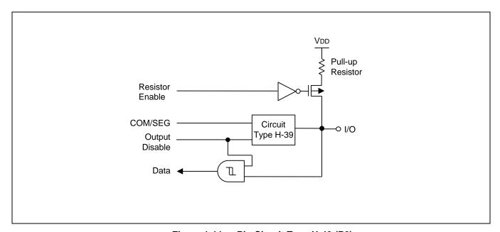
Figure 1-11 Pin Circuit Type H-43 (P2)
