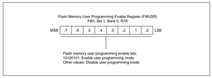
Figure 21-2 Flash Memory User Programming Enable Register (FMUSR)
