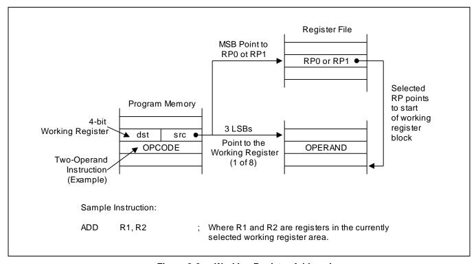
Figure 3-2 Working Register Addressing
