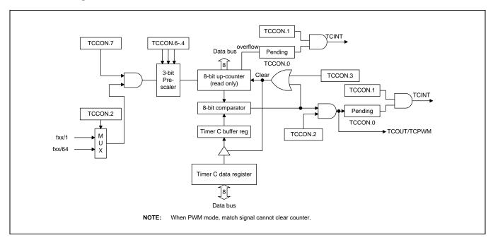
Figure 12-2 Timer C Function Block Diagram
