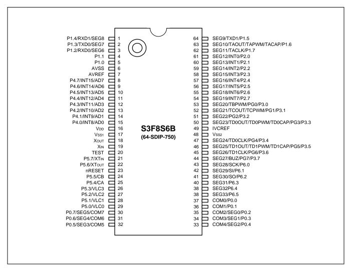
Figure 24-3 S3F8S6B Pin Assignments (64-SDIP-750)
