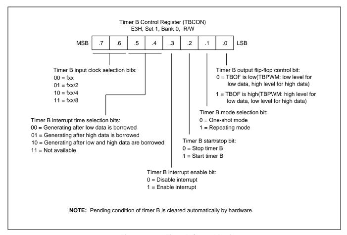
Figure 11-6 Timer B Control Register
