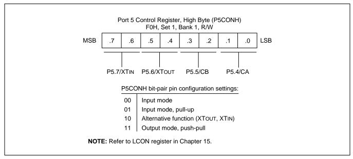
Figure 9-23 Port 5 High-Byte Control Register (P5CONH)
