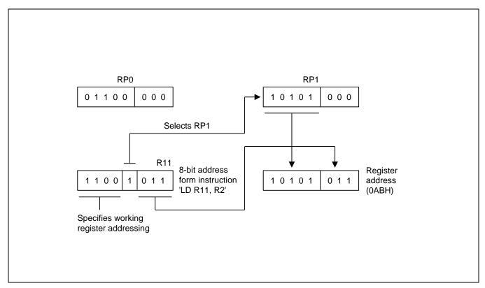
Figure 2-15 8-bit Working Register Addressing Example
