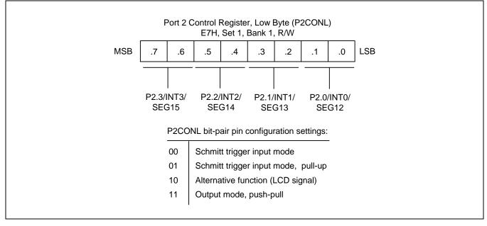
Figure 9-9 Port 2 Low-Byte Control Register (P2CONL)
