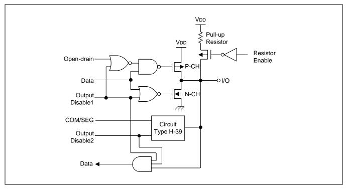
Figure 1-13 Pin Circuit Type H-42 (P1, P3, P6)
