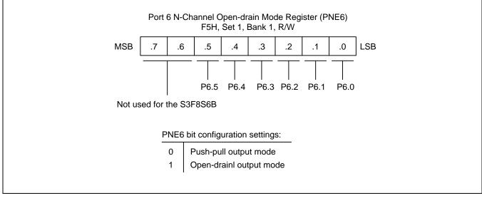
Figure 9-28 Port 6 N-Channel Open-drain Mode Register (PNE6)
