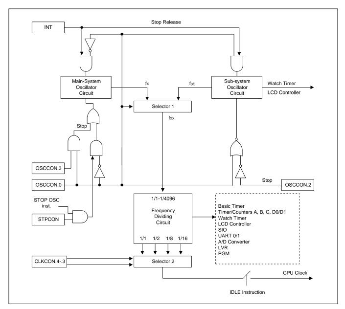
Figure 7-6 System Clock Circuit Diagram
