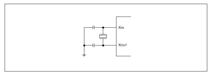
Figure 7-1 Crystal/Ceramic Oscillator (fX)
