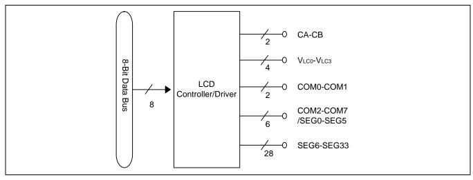
Figure 15-1 LCD Function Diagram
