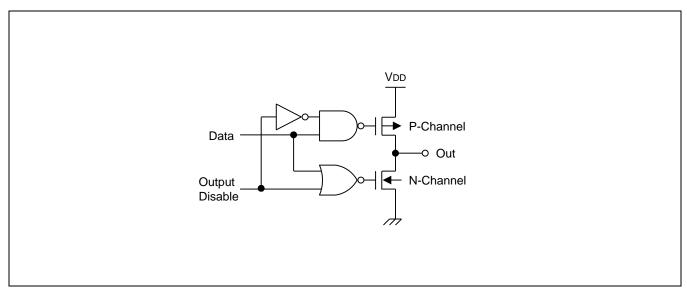
Figure 1-6 Pin Circuit Type C
