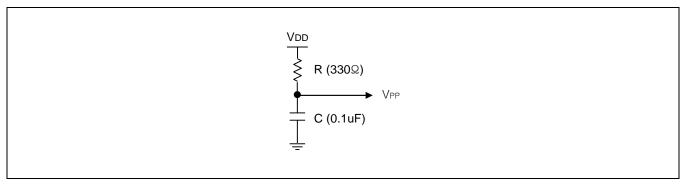
Figure 24-4 RC Delay Circuit
