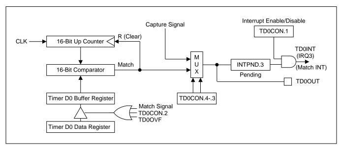
Figure 13-2 Simplified Timer D0 Function Diagram: Interval Timer Mode
