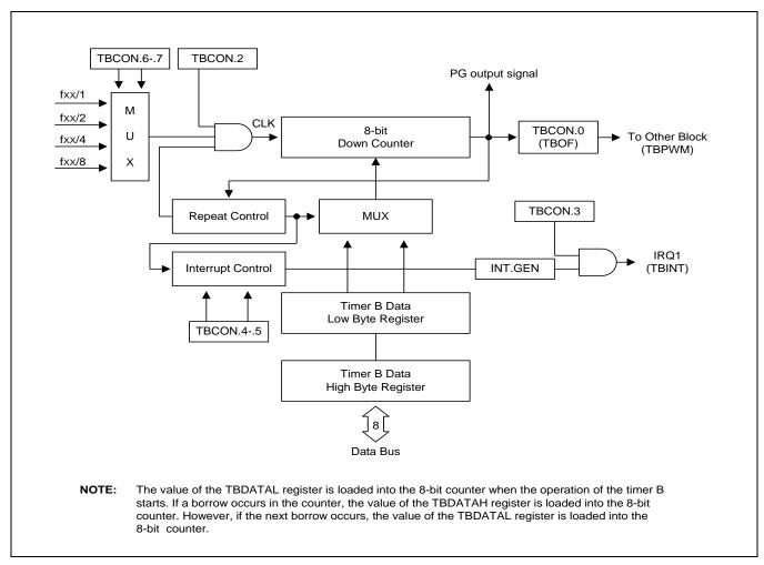
Figure 11-7 Timer B Functional Block Diagram
