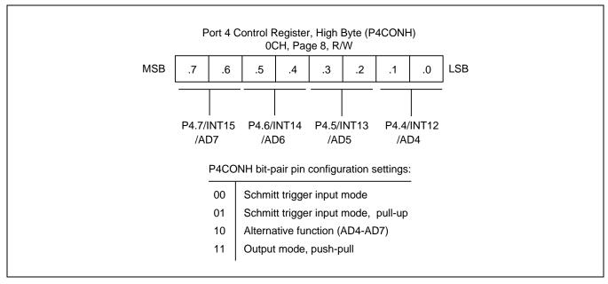
Figure 9-18 Port 4 High-Byte Control Register (P4CONH)
