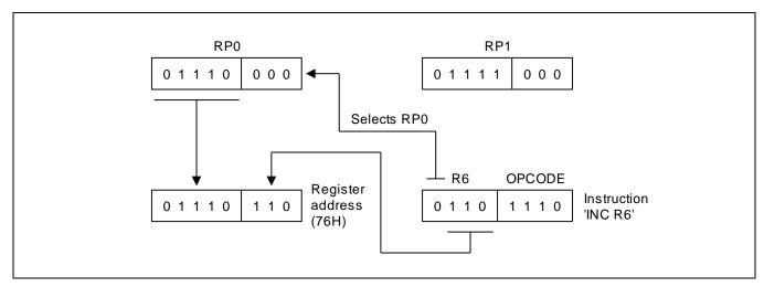
Figure 2-13 4-bit Working Register Addressing Example
