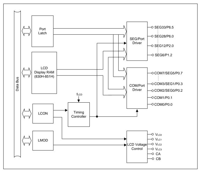
Figure 15-2 LCD Circuit Diagram
