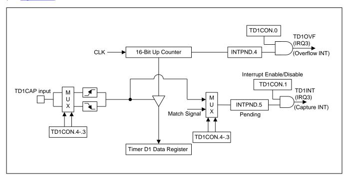
Figure 13-9 Simplified Timer D1 Function Diagram: Capture Mode
