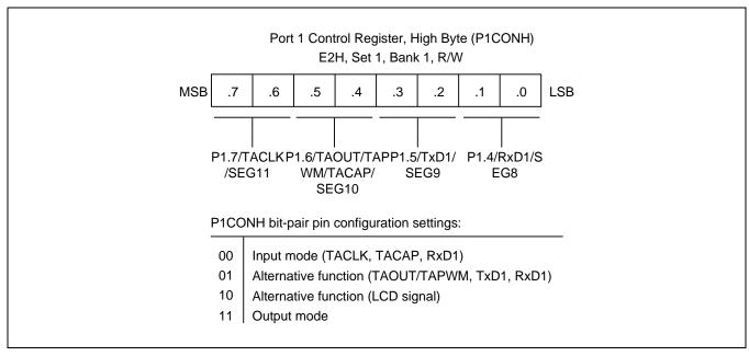
Figure 9-4 Port 1 High-Byte Control Register (P1CONH)
