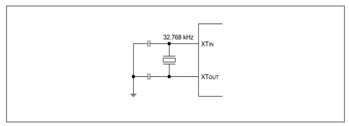
Figure 7-4 Crystal Oscillator (fxt)
