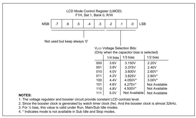
Figure 15-5 LCD Mode Control Register (LMOD)
