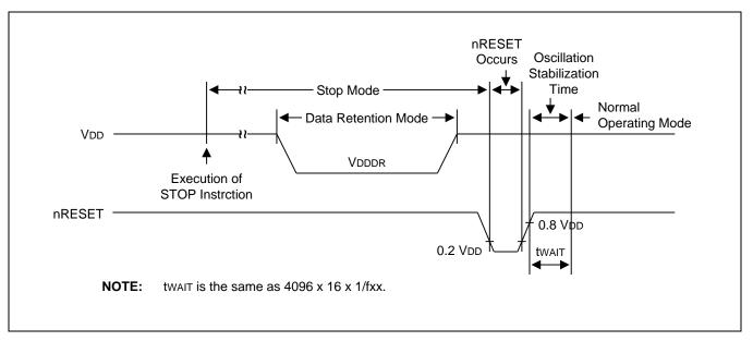
Figure 22-3 Stop Mode Release Timing Initiated by nRESET
