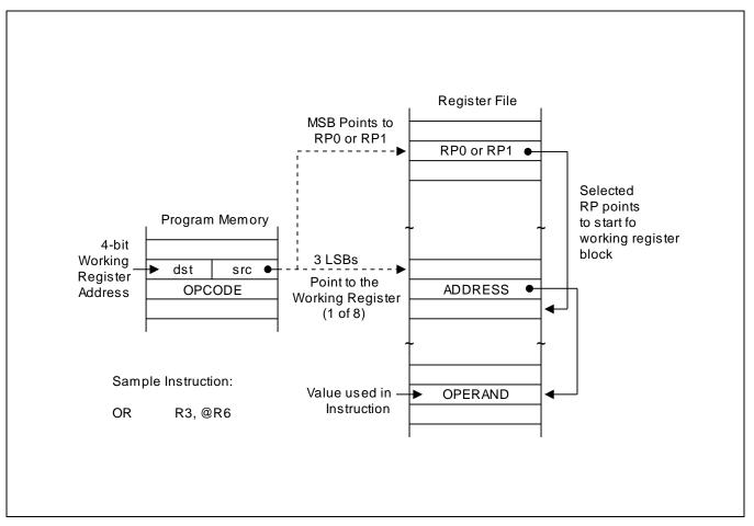
Figure 3-5 Indirect Working Register Addressing to Register File
