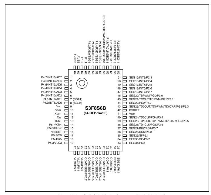
Figure 1-3 S3F8S6B Pin Assignments (64-QFP-1420F)
