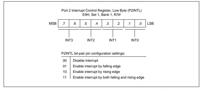
Figure 9-11 Port 2 Low-Byte Interrupt Control Register (P2INTL)
