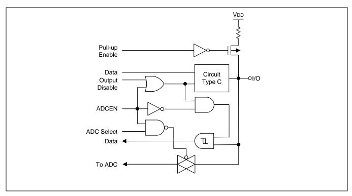
Figure 1-8 Pin Circuit Type F-16 (P4)
