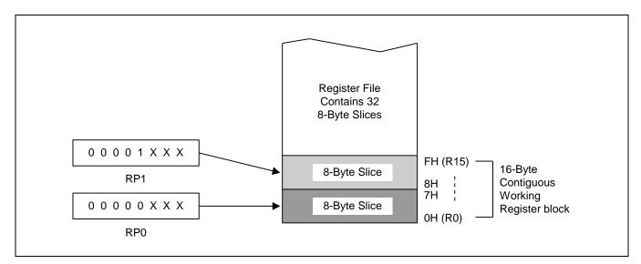
Figure 2-7 Contiguous 16 byte Working Register Block
