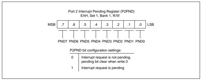
Figure 9-12 Port 2 Interrupt Pending Register (P2PND)
