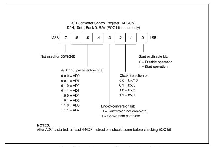
Figure 16-1 A/D Converter Control Register (ADCON)
