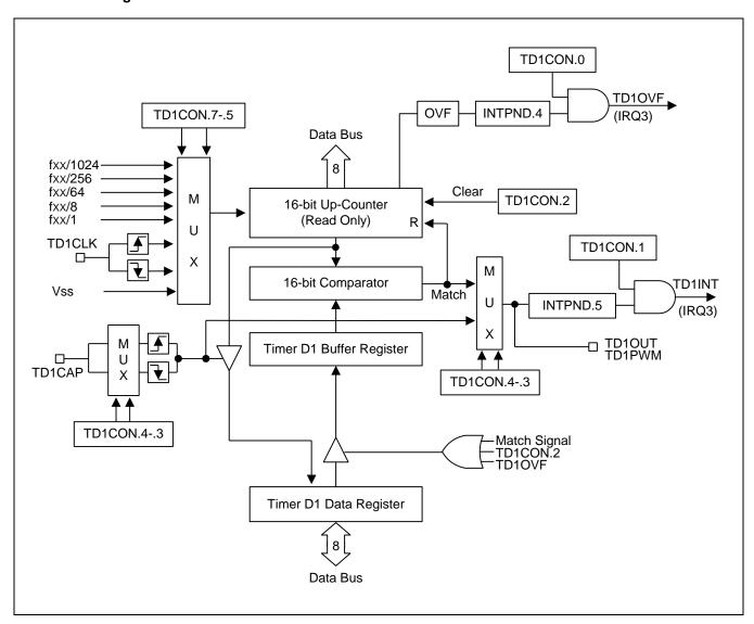
Figure 13-10 Timer D1 Functional Block Diagram
