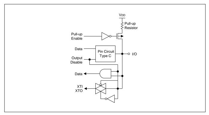
Figure 1-7 Pin Circuit Type D-2 (P5.6 – P5.7)
