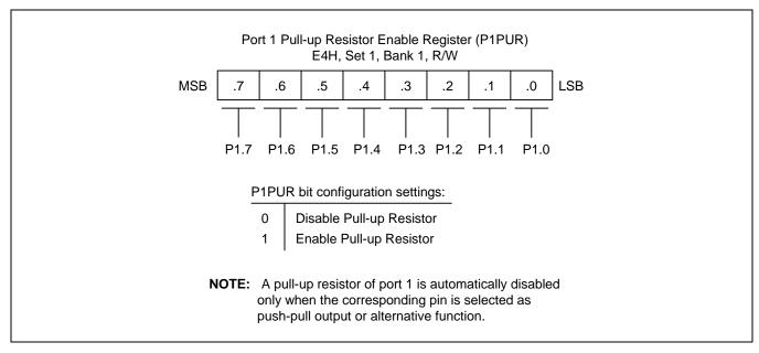
Figure 9-6 Port 1 Pull-up Resistor Enable Register (P1PUR)
