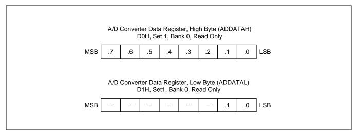
Figure 16-2 A/D Converter Data Register (ADDATAH/L)
