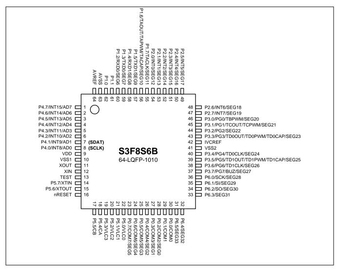
Figure 24-2 S3F8S6B Pin Assignments (64-LQFP-1010)
