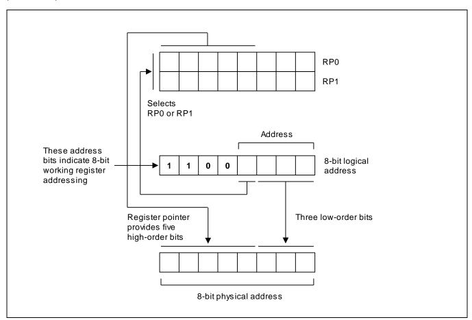
Figure 2-14 8-bit Working Register Addressing
