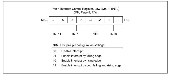
Figure 9-21 Port 4 Low-Byte Interrupt Control Register (P4INTL)
