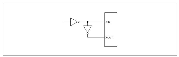
Figure 7-2 External Oscillator (fX)
