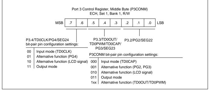
Figure 9-14 Port 3 Middle-Byte Control Register (P3CONM)
