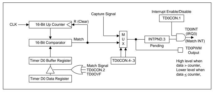
Figure 13-3 Simplified Timer D0 Function Diagram: PWM Mode
