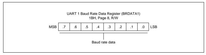
Figure 19-4 UART 1 Baud Rate Data Register (BRDATA1)
