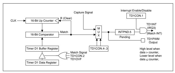
Figure 13-8 Simplified Timer D1 Function Diagram: PWM Mode
