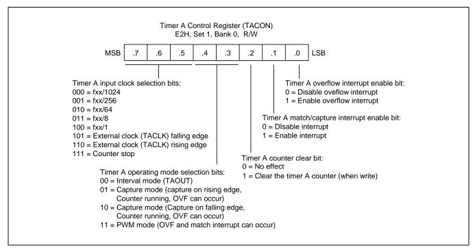
Figure 11-1 Timer A Control Register (TACON)
