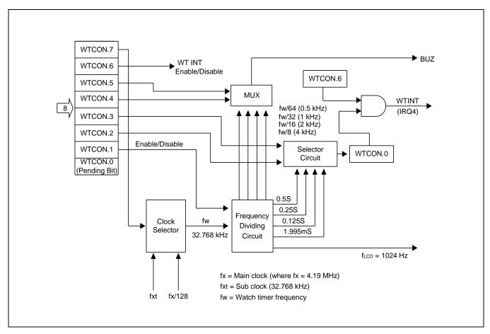
Figure 14-2 Watch Timer Circuit Diagram
