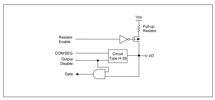
Figure 1-12 Pin Circuit Type H-44 (P0)
