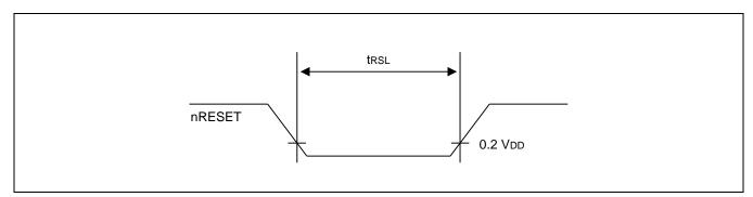
Figure 22-2 Input Timing for nRESET
