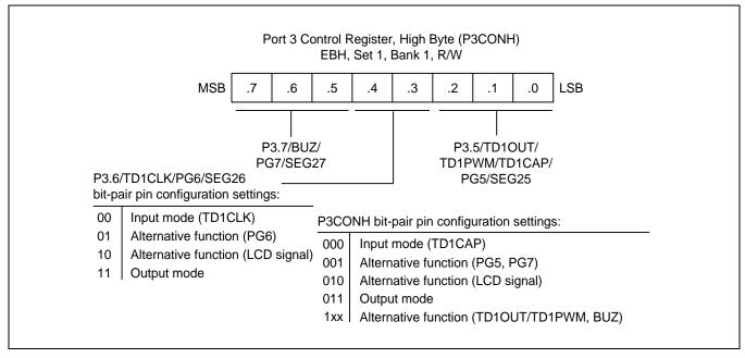
Figure 9-13 Port 3 High-Byte Control Register (P3CONH)
