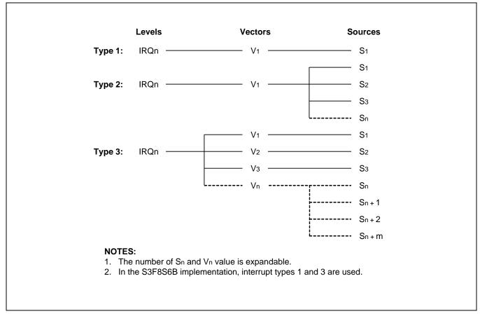
Figure 5-1 S3C8-Series Interrupt Types
