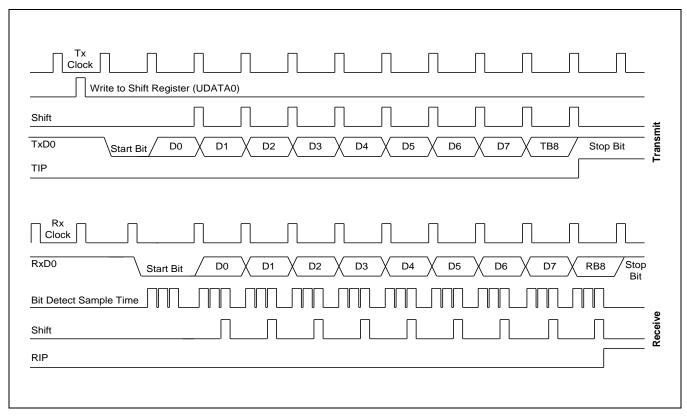
Figure 18-9 Timing Diagram for Serial Port Mode 3 Operation
