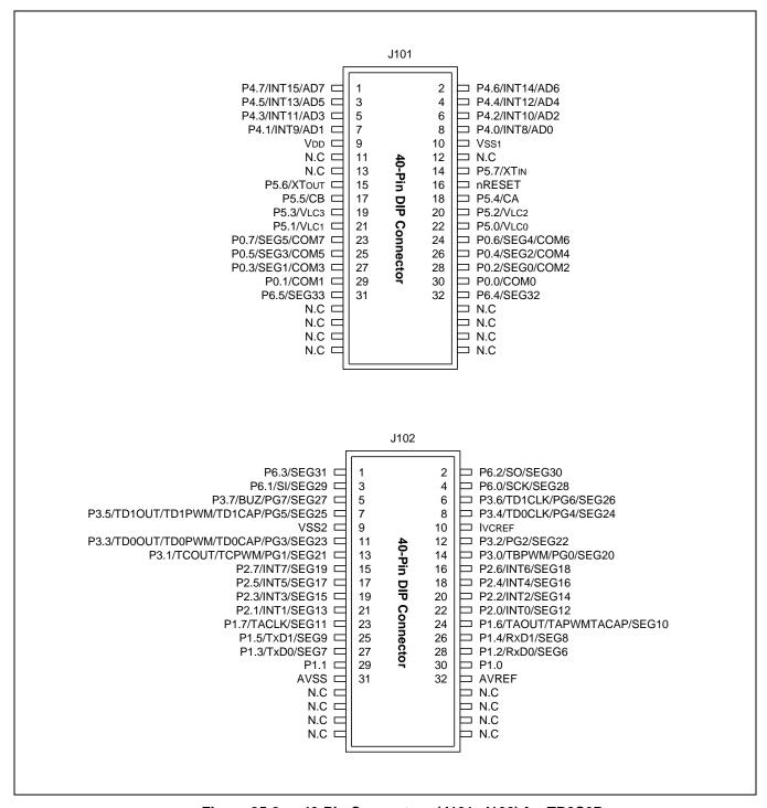
Figure 25-3 40-Pin Connectors (J101, J102) for TB8S6B
