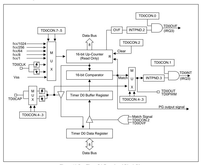
Figure 13-5 Timer D0 Functional Block Diagram
