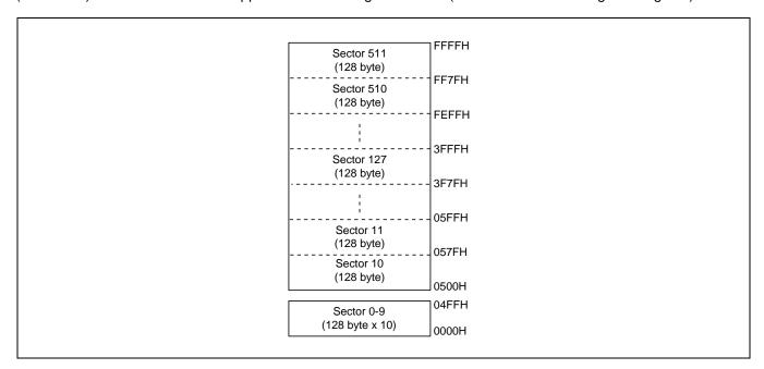
Figure 21-6 Sector Configurations in User Program Mode
