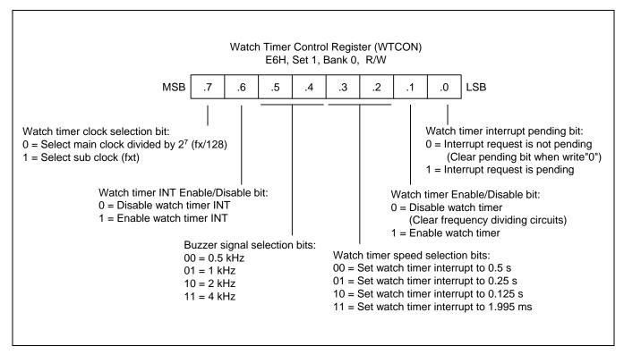
Figure 14-1 Watch Timer Control Register (WTCON)
