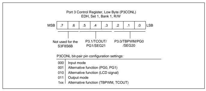
Figure 9-15 Port 3 Low-Byte Control Register (P3CONL)
