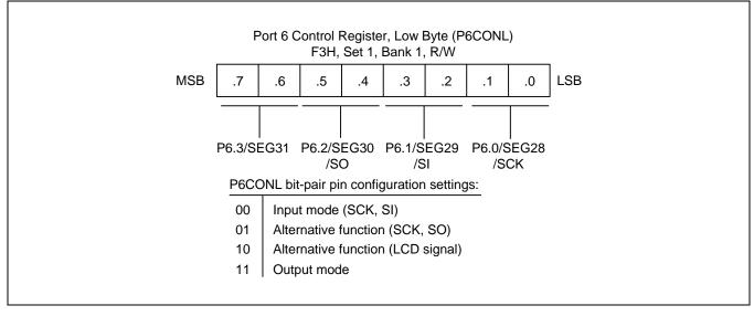
Figure 9-26 Port 6 Low-Byte Control Register (P6CONL)
