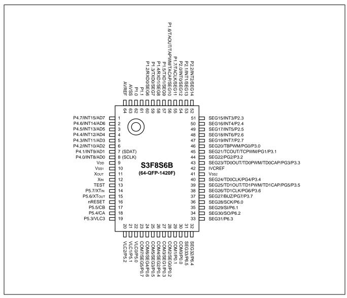
Figure 24-1 S3F8S6B Pin Assignments (64-QFP-1420F)
