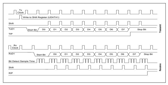
Figure 19-7 Timing Diagram for Serial Port Mode 1 Operation
