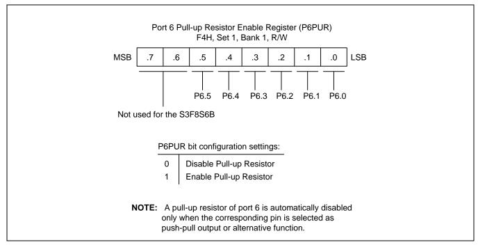
Figure 9-27 Port 6 Pull-up Resistor Enable Register (P6PUR)
