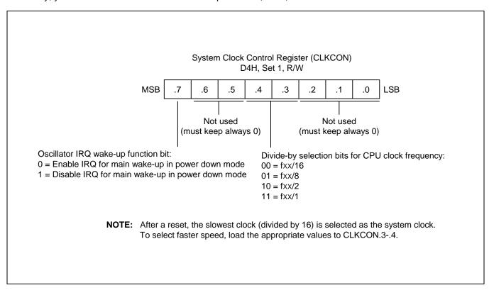
Figure 7-7 System Clock Control Register (CLKCON)
