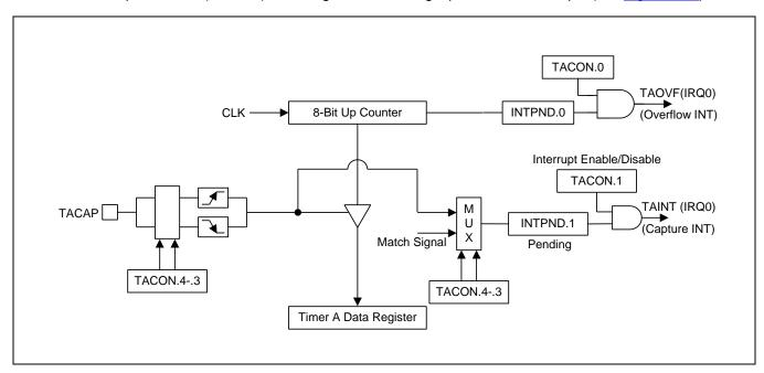
Figure 11-4 Simplified Timer A Function Diagram: Capture Mode
