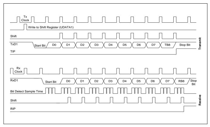
Figure 19-9 Timing Diagram for Serial Port Mode 3 Operation
