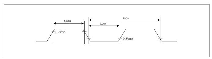
Figure 22-7 Waveform for UART Timing Characteristics
