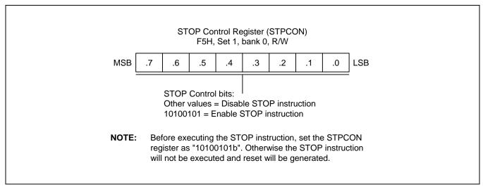
Figure 7-9 STOP Control Register (STPCON)
