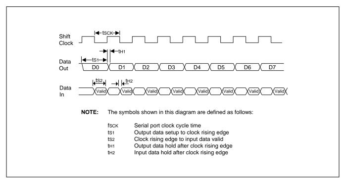
Figure 22-8 Timing Waveform for the UART Module
