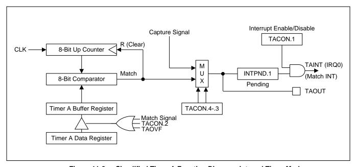
Figure 11-2 Simplified Timer A Function Diagram: Interval Timer Mode
