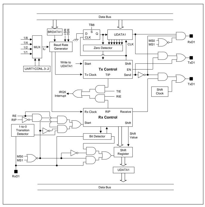
Figure 19-5 UART 1 Functional Block Diagram
