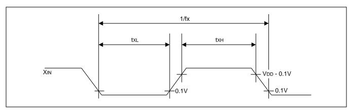
Figure 22-9 Clock Timing Measurement at XIN
