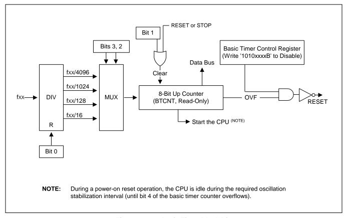
Figure 10-2 Basic Timer Block Diagram
