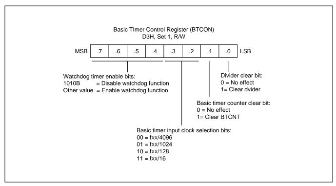
Figure 10-1 Basic Timer Control Register (BTCON)
