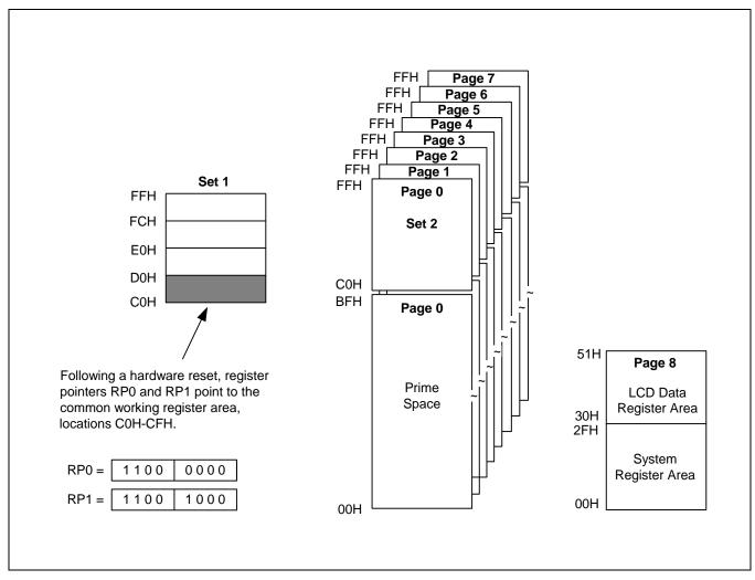
Figure 2-11 Common Working Register Area
