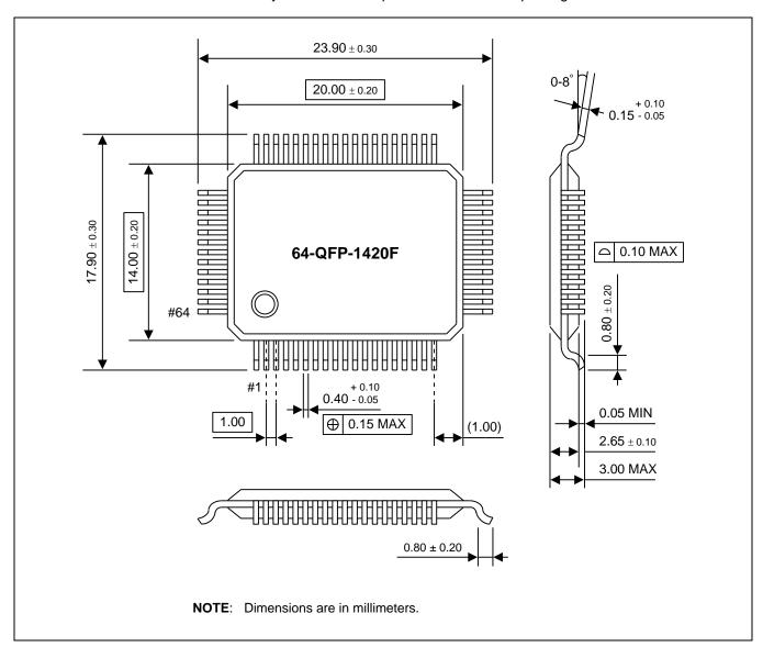
Figure 23-1 Package Dimensions (64-QFP-1420F)
