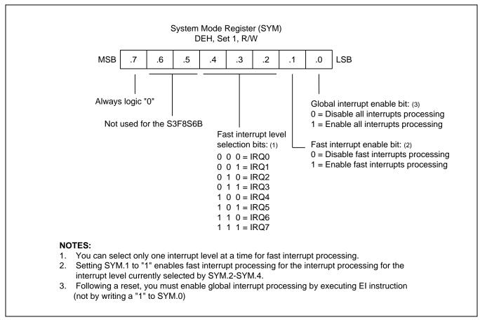
Figure 5-5 System Mode Register (SYM)
