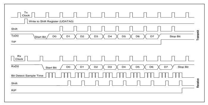
Figure 18-7 Timing Diagram for Serial Port Mode 1 Operation
