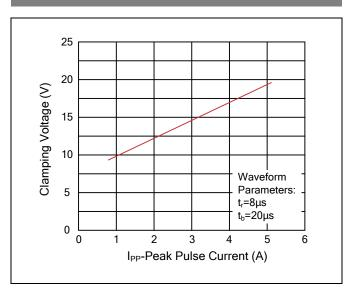
Figure 4. ESD Clamping(8kV Contact IEC61000-4-2)
