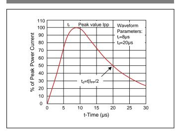
Figure 3. Non-Repetitive Peak Pulse vs. Pulse Time
