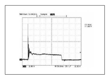
Figure 6. ESD Clamping(-8kV Contact IEC61000-4-2)
