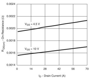
On-Resistance vs. Drain Current and Gate Voltage
