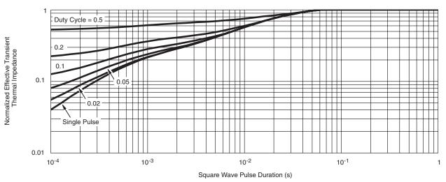
Normalized Thermal Transient Impedance, Junction-to-Case
