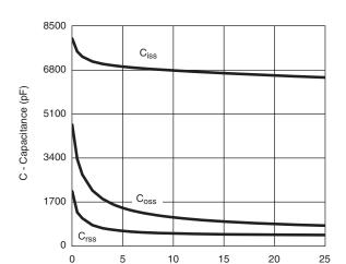
V<sub>DS</sub> - Drain-to-Source Voltage (V)
