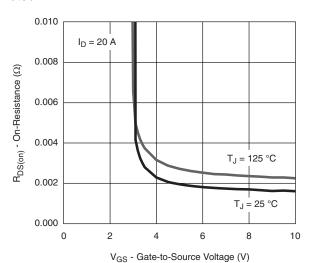
On-Resistance vs. Gate-to-Source Voltage
