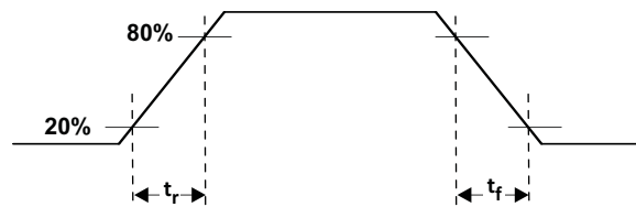
Figure 3. Output Rise and Fall Times
