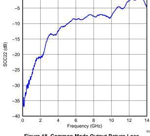
Figure 18. Common Mode Output Return Loss
