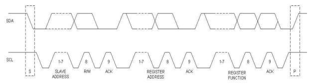
Figure 24. Two-wire Serial Interface Data Transfer
