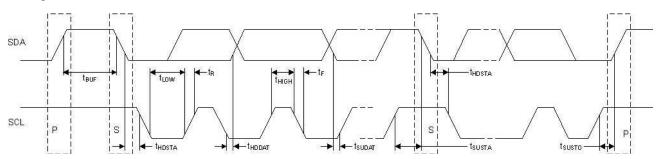
Figure 23. Two-wire Serial Interface Timing Diagram
