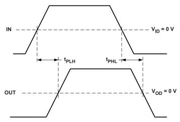
Figure 6. Propagation Delay Input to Output
