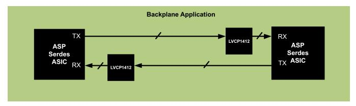
Figure 1. Typical Backplane Application – Trace Mode
