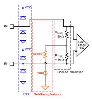
Figure 12. Equivalent Input Circuit Design
