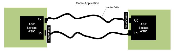
Figure 2. Typical Cable Application - Cable Mode
