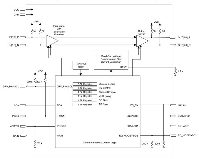
Figure 3. Simplified Block Diagram of the SN65LVCP1412
