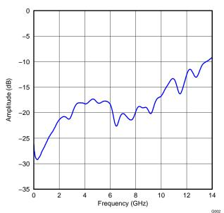
Figure 15. Differential Input Return Loss
