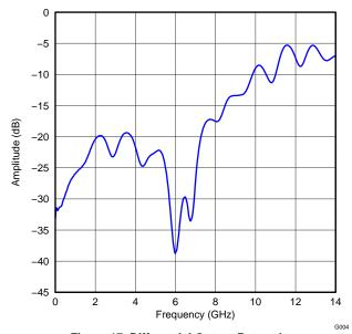
Figure 17. Differential Output Return Loss
