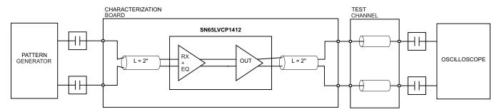
Figure 11. Transmit Side Performance Test Circuit
