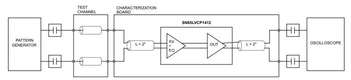
Figure 10. Receive Side Performance Test Circuit
