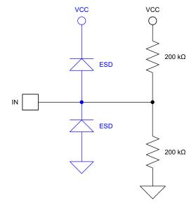
Figure 13. 3-Level Input Biasing Network
