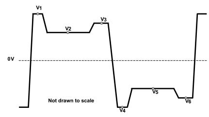
Figure 9. Vpre and Vpost (The test pattern is 1111111100000000 (8-1s, 8-0s))
