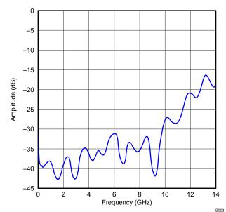
Figure 16. Differential to Common Mode Conversion
