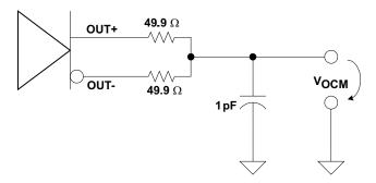
Figure 5. Common Mode Output Voltage Test Circuit
