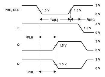
Figure 1. CLR and PRE Pulse Duration, CLR and PRE to Output Delay, and CLR and PRE to Latch-Enable Recovery Time
