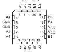
The output drive for each mode is determined by the high-drive (HD) control pin. When HD is high, the high drive is delivered by the totem-pole configuration, and when HD is low, the outputs are open drain. This meets the drive requirements as specified in the IEEE 1284-I (level-1 type) and the IEEE 1284-II (level-2 type) parallel peripheral-interface specification.
