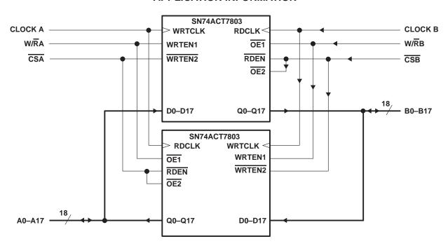
Figure 9. Bidirectional Configuration
