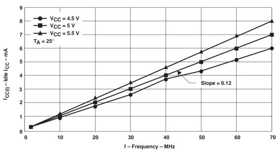
Figure 8. SN74ACT7803 Idle I<sub>CC</sub> With RDCLK or WRTCLK Switching
