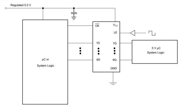
Figure 4. Typical Application Schematic
