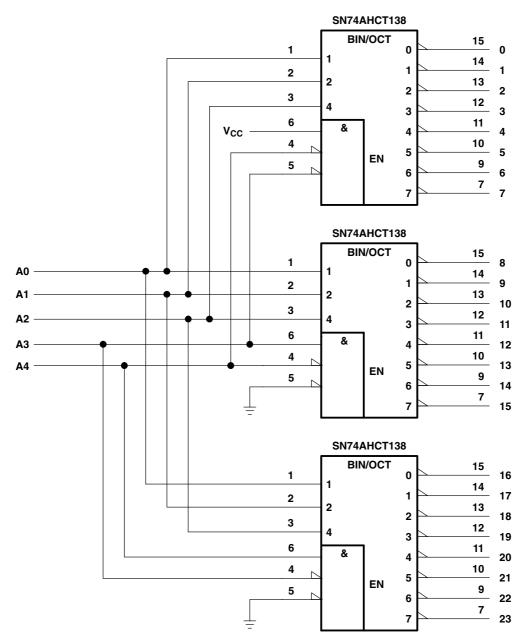
Figure 2. 24-Bit Decoding Scheme
