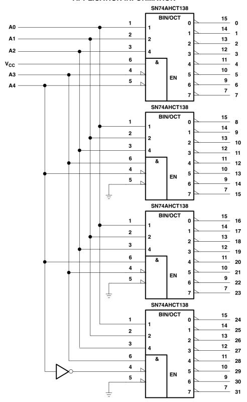
Figure 3. 32-Bit Decoding Scheme
