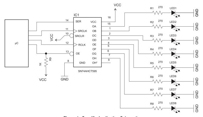
Figure 4. Specific Application Schematic
