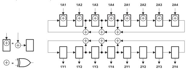
Figure 7. 8-Bit PSA/PRPG Configuration
