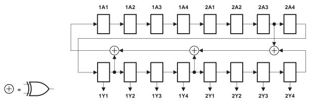
Figure 5. 16-Bit PRPG Configuration
