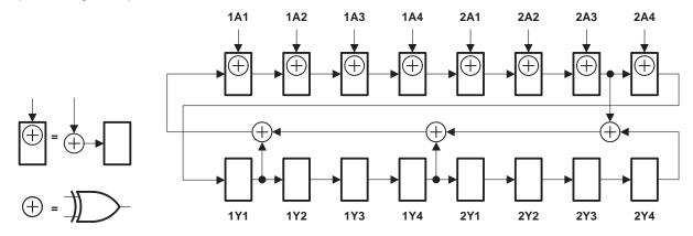
Figure 6. 16-Bit PSA Configuration
