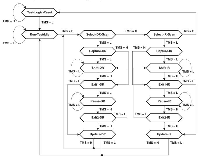
Figure 1. TAP-Controller State Diagram
