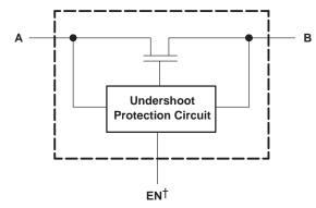
†EN is the internal enable signal applied to the switch.
