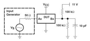
Figure 8-1. Device Test Setup
