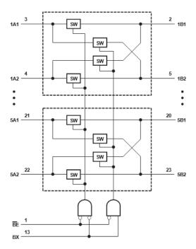
Logic Diagram (Positive Logic)
