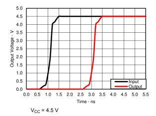
Figure 10-2. Propagation Delay (t<sub>pd</sub>) Simulation Results
