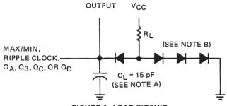
FIGURE 1-LOAD CIRCUIT FOR SWITCHING TIME MEASUREMENT
