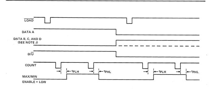
NOTE J: Data inputs B and C are shown by the dashed line for the '190 and 'LS190 and the solid line for the '191 and 'LS191: Data input D is shown by the solid line for both devices.
