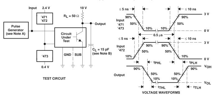
NOTES: A. The pulse generator has the following characteristics: PRR  $\leq$  1 MHz,  $Z_{\mbox{\scriptsize O}}\approx$  50  $\Omega$
