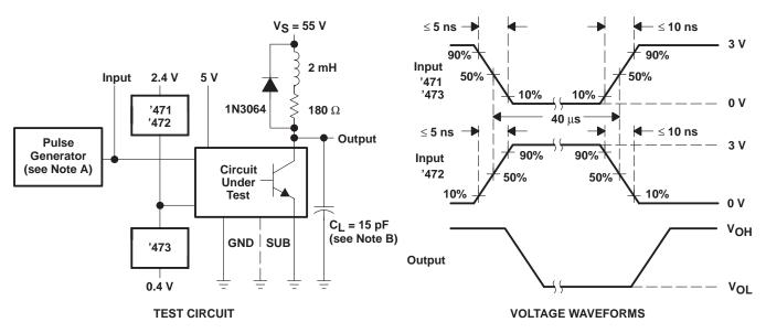
NOTES: A. The pulse generator has the following characteristics: PRR  $\leq$  12.5 kHz,  $Z_O\approx$  50  $\Omega$
