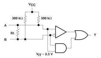
Figure 9. Open-Circuit Fail Safe of the LVDS Receiver
