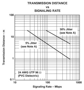
NOTE A: This parameter is the percentage of distortion of the unit interval (UI) with a pseudorandom data pattern.
