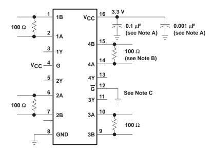
NOTES: A. Place a 0.1 µF and a 0.001 µF Z5U ceramic, mica or polystyrene dielectric, 0805 size, chip capacitor between V<sub>CC</sub> and the ground plane. The capacitors should be located as close as possible to the device terminals.
