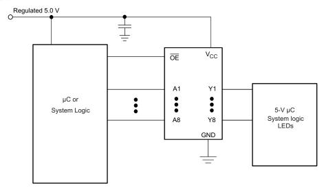
Figure 3. Typical Application Schematic
