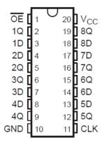
J, W, DB, DW, N, NS, or PW package 20-Pin CDIP, CFP, SSOP, SOIC, PDIP, SO, or TSSOP Top View
