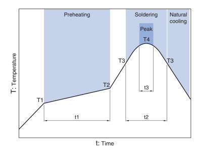
Preheating Soldering Peak Temp. Time Temp. Time Temp. Time T1 T2 T4 Т3 t3 150°C 180°C 120s 230°C 260°C 10s max. 30s
