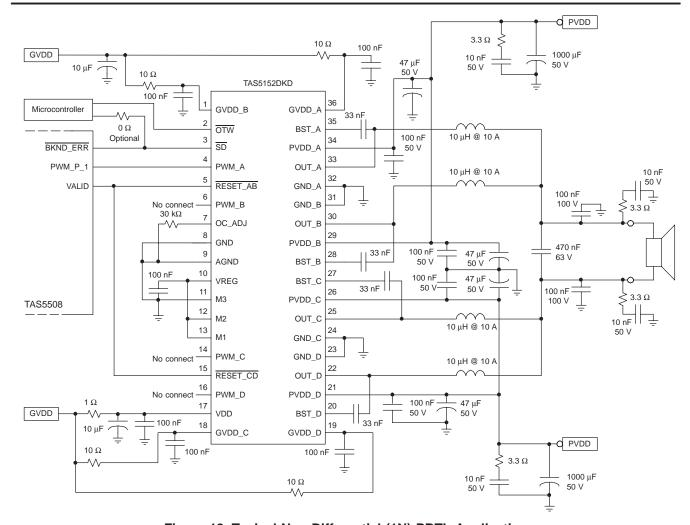
Figure 18. Typical Non-Differential (1N) PBTL Application
