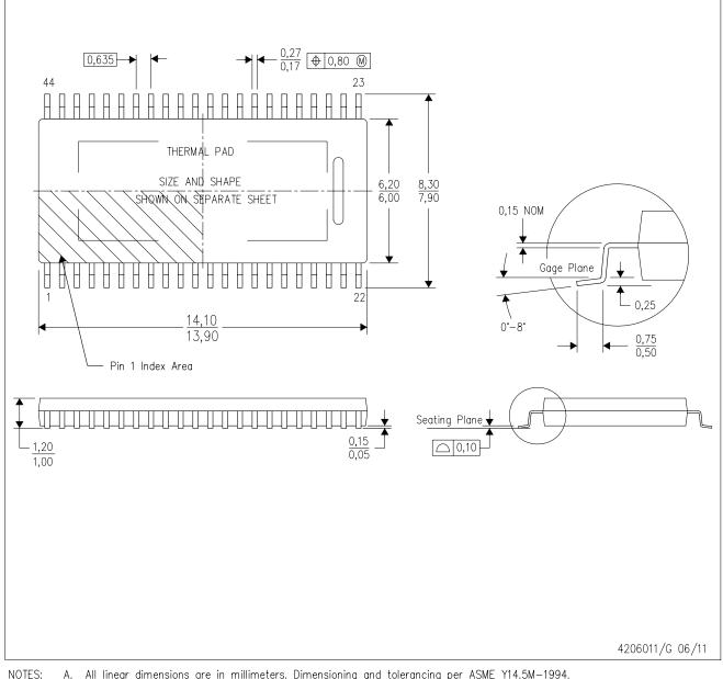
A. All linear dimensions are in millimeters. Dimensioning and tolerancing per ASME Y14.5M-1994. B. This drawing is subject to change without notice.
