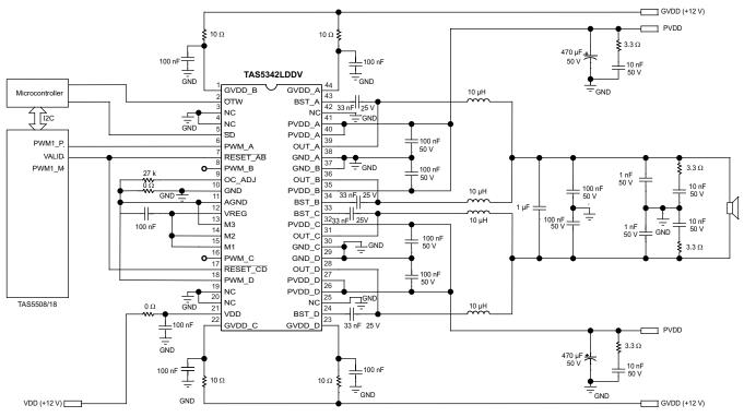
Figure 18. Typical Non-Differential (1N) PBTL Application
