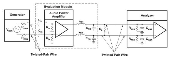
Figure 25. Differential Input, BTL Output Measurement Circuit
