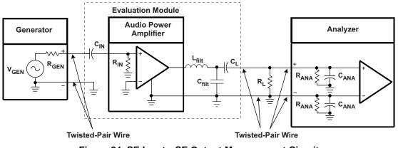
Figure 24. SE Input—SE Output Measurement Circuit
