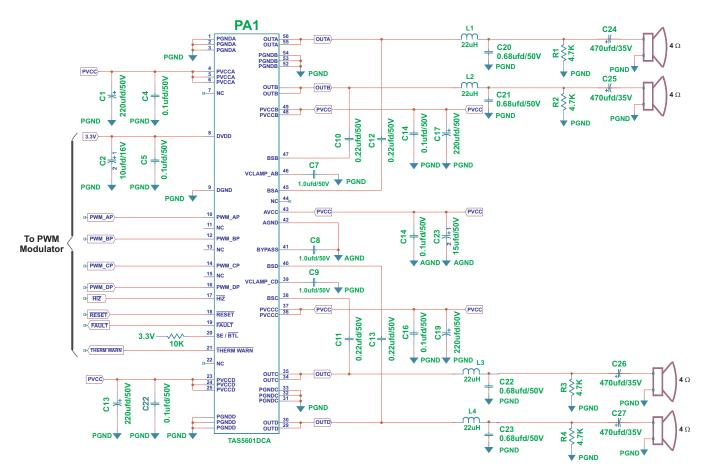
Figure 2. Single Ended (SE) Application Schematic
