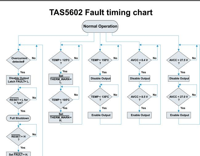
Figure 20. Device Protection Flow Chart
