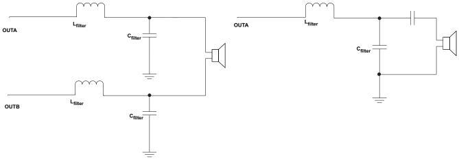
Figure 21. BTL Filter Configuration
