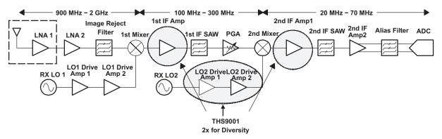
Figure 22. Example Dual Conversion Receiver Architecture
