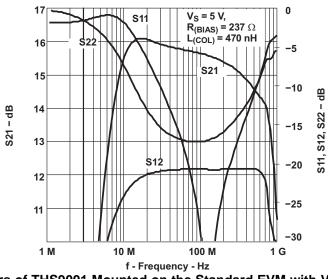
Figure 20. S-Parameters of THS9001 Mounted on the Standard EVM with V<sub>S</sub> = 5 V, R<sub>(BIAS)</sub> = 237  $\Omega$ , and L<sub>(COL)</sub> = 470 nH
