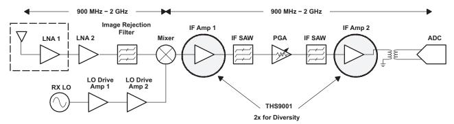
Figure 21. Example Single Conversion Receiver Architecture
