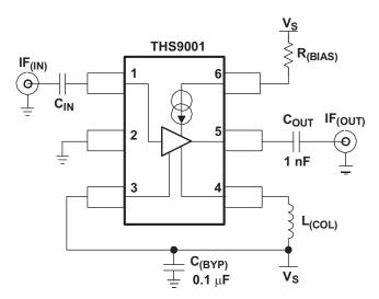
Figure 25. THS9000 Recommended Circuit (used for all tests)
