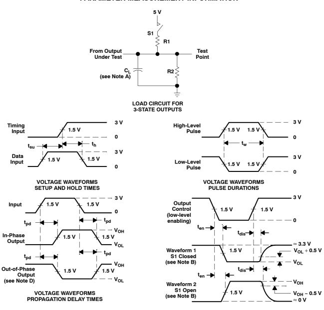
NOTES: A. C<sub>L</sub> includes probe and jig capacitance and is 50 pF for t<sub>pd</sub> and t<sub>en</sub>, 5 pF for t<sub>dis</sub>.
