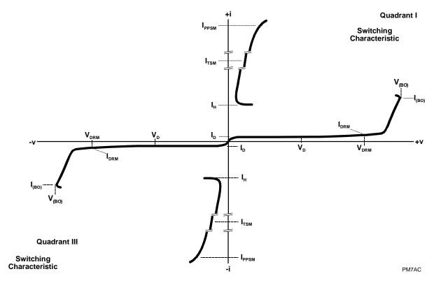
Figure 1. Voltage-Current Characteristic for any Terminal Pair
