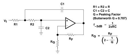
Figure 39. 2-Pole Low-Pass Sallen-Key Filter
