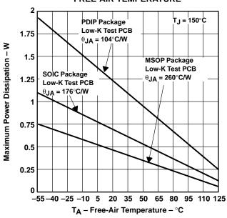
NOTE A: Results are with no air flow and using JEDEC Standard Low-K test PCB.
