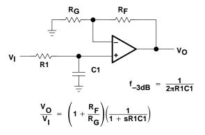
Figure 38. Single-Pole Low-Pass Filter
