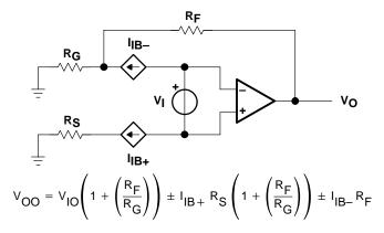
Figure 37. Output Offset Voltage Model
