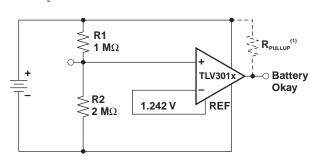
When the battery voltage drops below 1.9 V, the Battery Okay output goes low.
