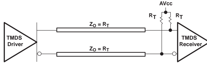
Figure 1. Termination for TMS Output Driver
