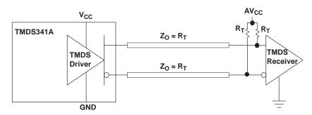
Figure 35. TMDS Driver and Termination Circuit
