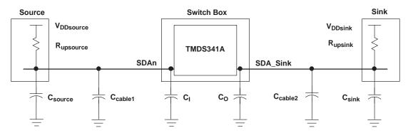
Figure 40. DDC Link from Source to Sink With External Switch Box
