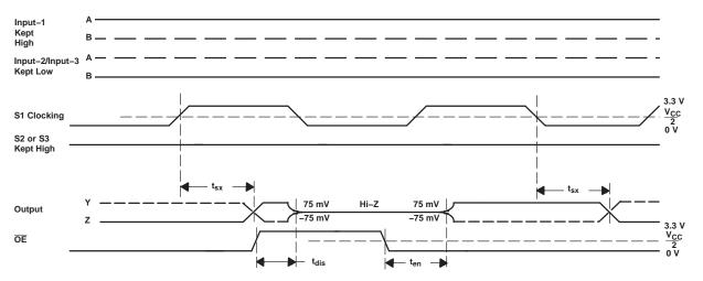
**Figure 6. TMDS Outputs Control Timing Definitions**
