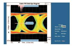
Figure 39. Eye Diagram Recovered by TMDS341A vs TP2
