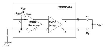
Figure 34. TMDS Input Fail-Safe Recommendation
