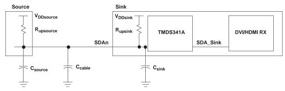
Figure 41. DDC Link From Source to Sink Without External Switch Box
