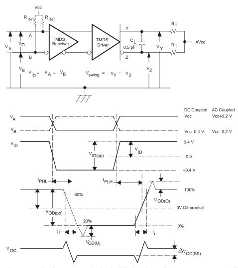
NOTE: All input pulses are supplied by a generator having the following characteristics:  $t_r$  or  $t_f$  < 100 ps, 100 MHz from Agilent 81250.  $C_L$  includes instrumentation and fixture capacitance within 0.06 m of the D.U.T. Measurement equipment provides a bandwidth of 20 GHz minimum.
