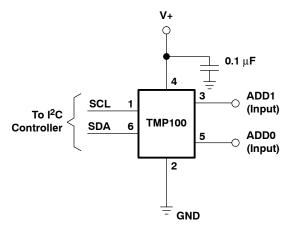
NOTE 2: SCL and SDA require pullup resistors for I<sup>2</sup>C bus applications.
