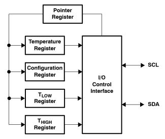
Figure 2. Internal Register Structure of TMP100 and TMP101
