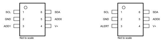
Figure 5-1. TMP100-Q1 DBV Package 6-Pin SOT-23 Figure 5-2. TMP101-Q1 DBV Package 6-Pin SOT-23 **Top View Top View**
