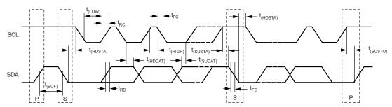
Figure 7-3. I<sup>2</sup>C Timing Diagram
