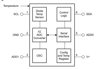
Figure 7-1. TMP100-Q1 Block Diagram
