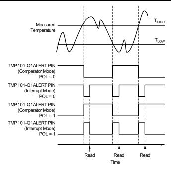
Figure 7-8. Output Transfer Function Diagrams
