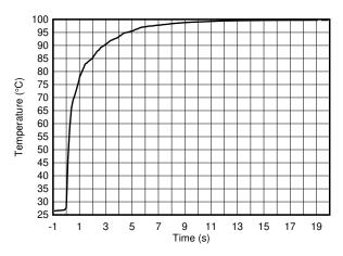
Figure 8-3. Temperature Step Response
