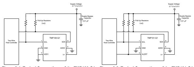
Figure 8-1. Typical Connections of the TMP100-Q1 Figure 8-2. Typical Connections of the TMP101-Q1
