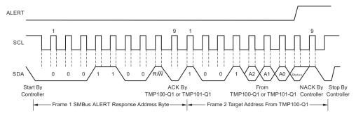
Figure 7-6. Timing Diagram for SMBus ALERT
