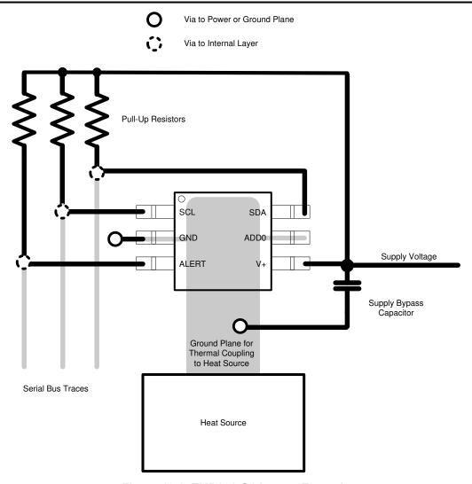
Figure 10-2. TMP101-Q1 Layout Example
