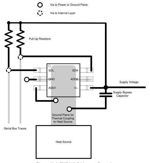
Figure 10-1. TMP100-Q1 Layout Example
