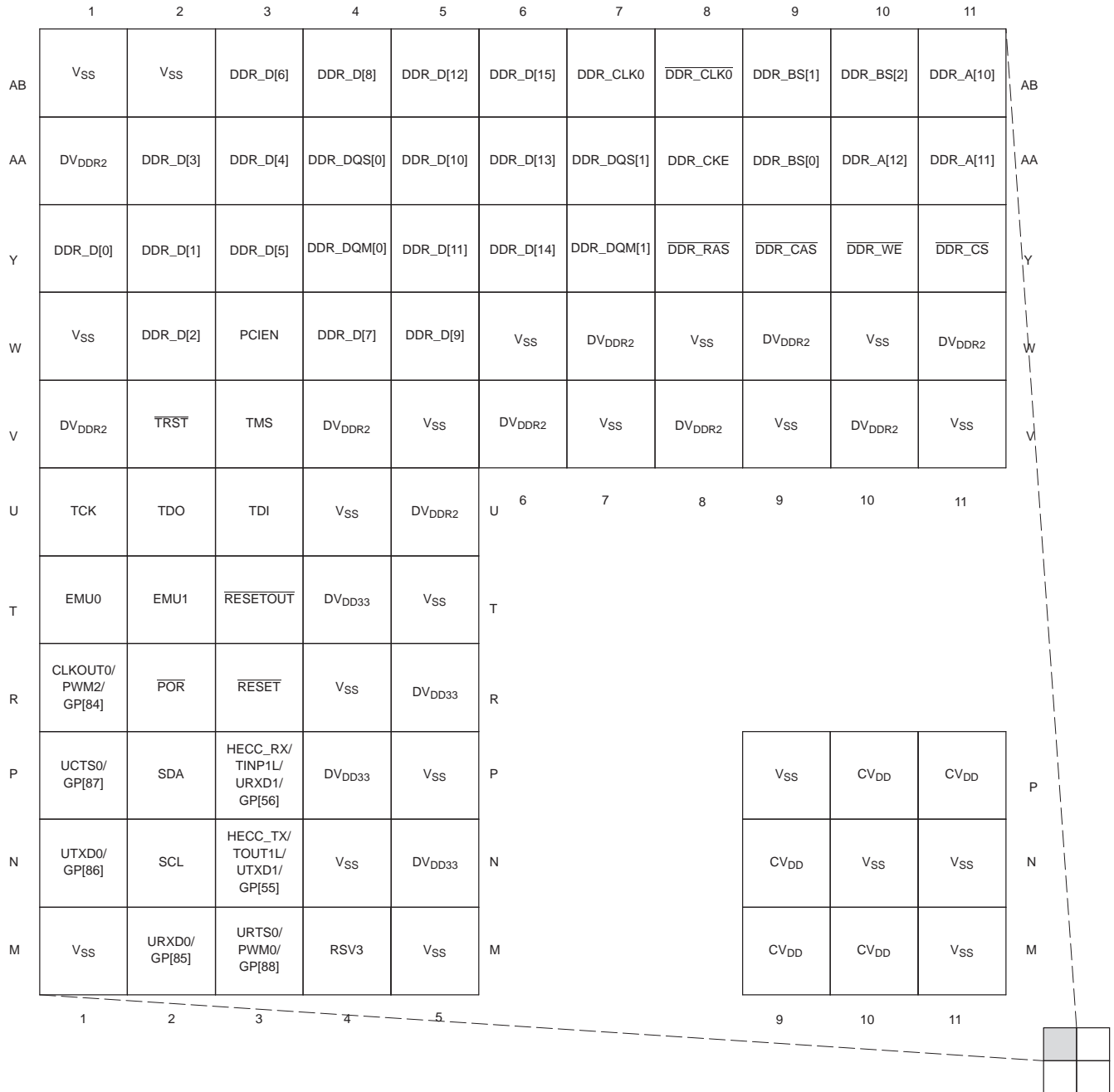
Figure 2-6. ZDU Pin Map [Quadrant A]
