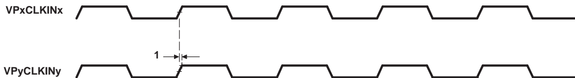
Figure 5-57. Video Port Dual-Display Sync Timing
