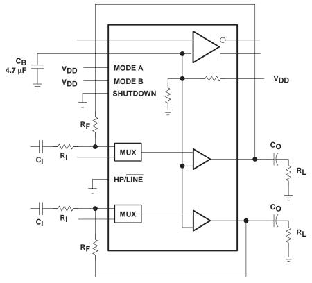
Figure 2. SE Test Circuit
