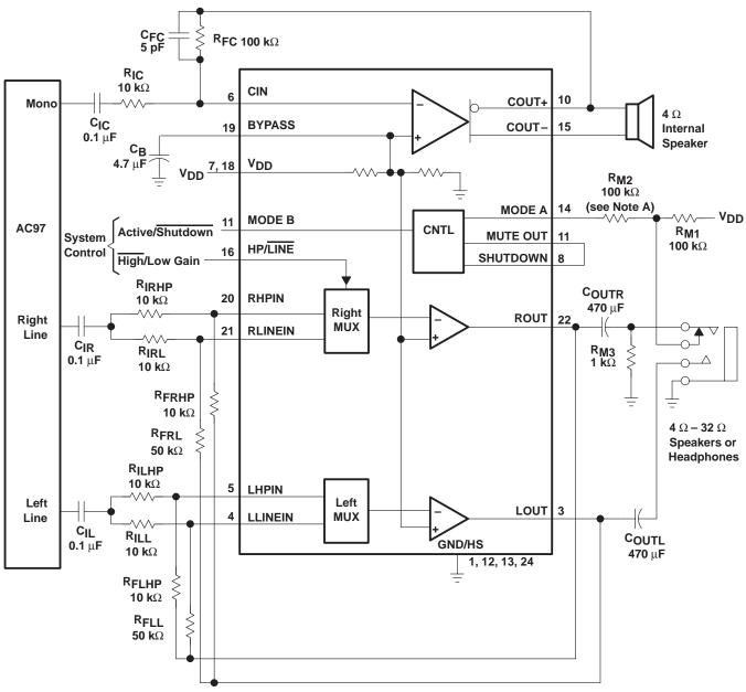
NOTE A: This connection is for ultralow current in shutdown mode.
