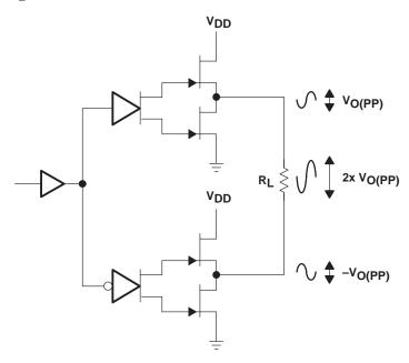
Figure 59. Bridge-Tied Load Configuration
