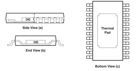
Figure 58. Views of Thermally Enhanced PWP Package
