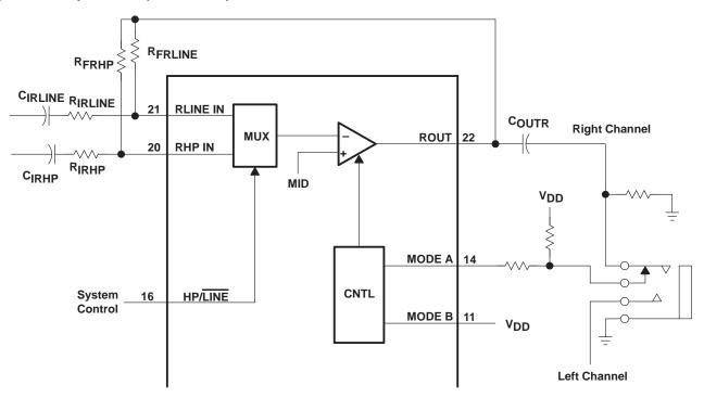
Figure 64. TPA0103 Example Input MUX Circuit
