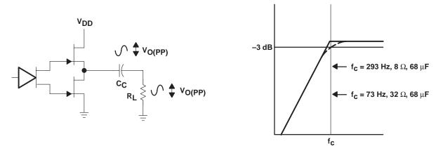
Figure 60. Single-Ended Configuration and Frequency Response
