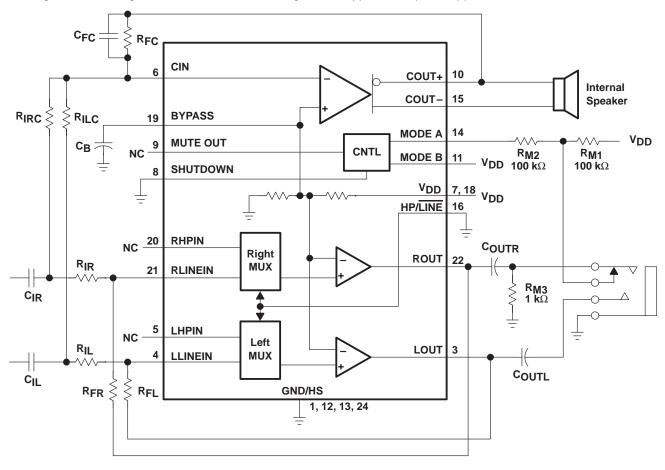
Figure 62. TPA0103 Minimum Configuration Application Circuit
