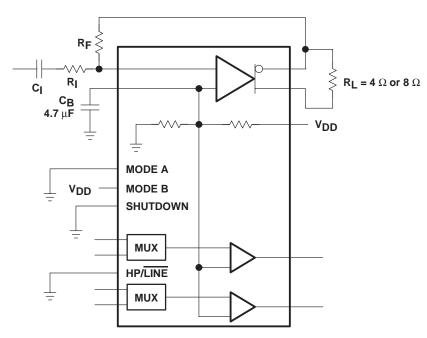
Figure 1. BTL Test Circuit
