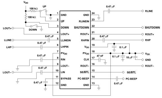
Figure 29. Typical TPA0152 Application Circuit
