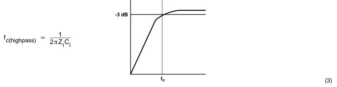
The value of  $C_i$  is important to consider as it directly affects the bass (low frequency) performance of the circuit. Consider the example where  $Z_i$  is 15 k $\Omega$  (see Figure 28) and the specification calls for a flat-bass response down to 40 Hz. Equation 3 is reconfigured as Equation 4.
