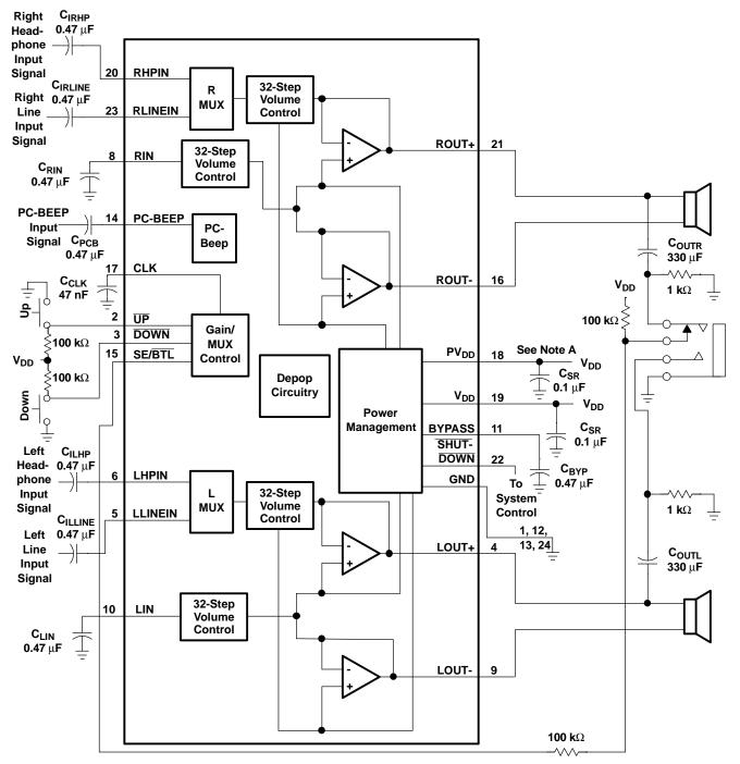
NOTE: A 0.1-µF ceramic capacitor should be placed as close as possible to the IC. For filtering lower-frequency noise signals, a larger electrolytic capacitor of 10 µF or greater should be placed near the audio power amplifier.
