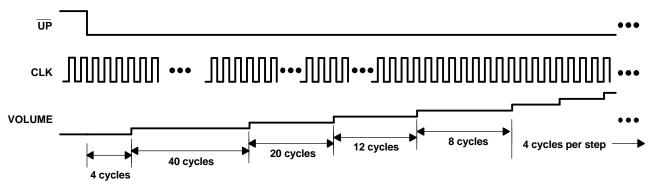
Figure 32. Internal Clock Timing Diagram
