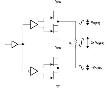
Figure 35. Bridge-Tied Load Configuration
