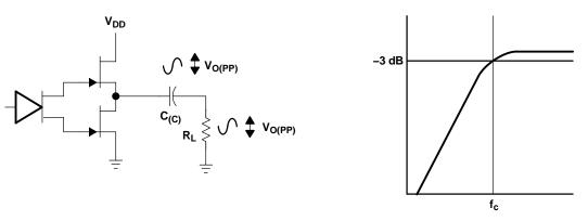
Figure 36. Single-Ended Configuration and Frequency Response
