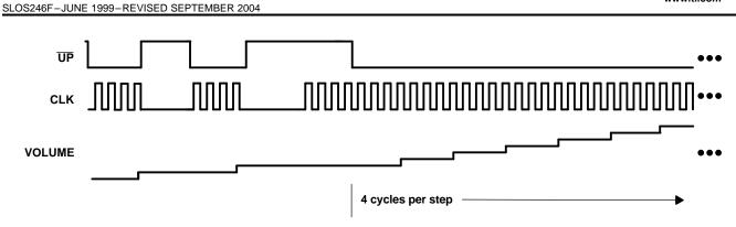
Figure 33. External Clock (4 Cycles Per Volume Change)
