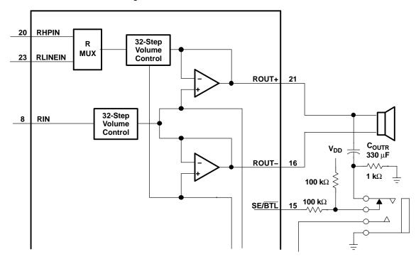
Figure 38. TPA0152 Resistor Divider Network Circuit
