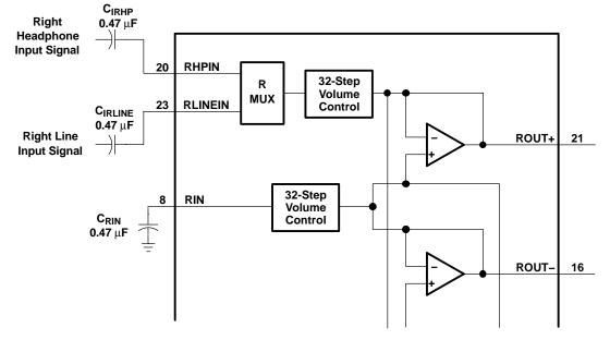
Figure 39. TPA0152 Example Input MUX Circuit
