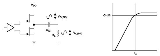
Figure 37. Single-Ended Configuration and Frequency Response
