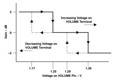
Figure 33. DC Volume Control Operation
