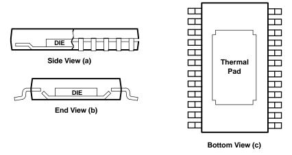
Figure 30. Views of Thermally Enhanced PWP Package
