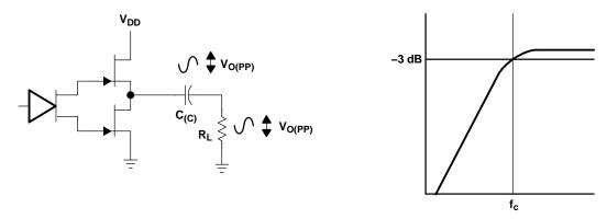
Figure 36. Single-Ended Configuration and Frequency Response
