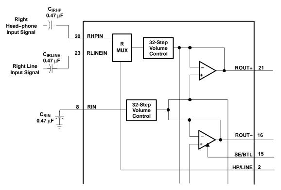
Figure 40. TPA0232 Example Input MUX Circuit
