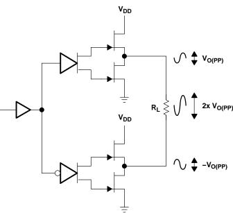
Figure 35. Bridge-Tied Load Configuration
