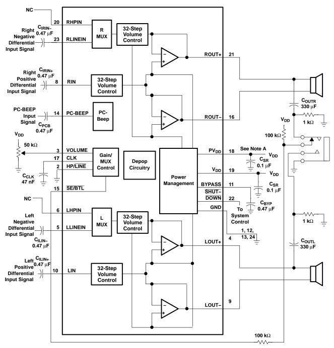
A. A 0.1-μF ceramic capacitor should be placed as close as possible to the IC. For filtering lower-frequency noise signals, a larger electrolytic capacitor of 10 μF or greater should be placed near the audio power amplifier.
