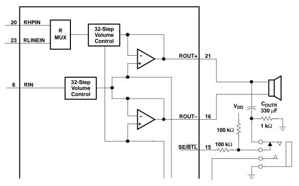
Figure 39. TPA0232 Resistor Divider Network Circuit
