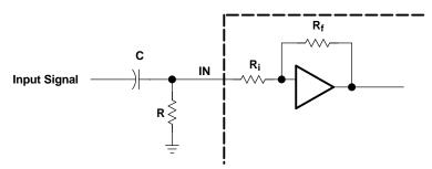
Figure 34. Resistor on Input for Cut-Off Frequency
