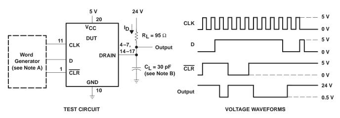
Figure 1. Resistive Load Normal Operation
