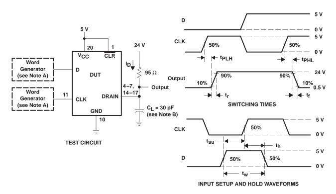
Figure 2. Test Circuit, Switching Times, and Voltage Waveforms
