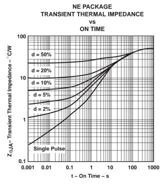
The single-pulse curve represents measured data. The curves for various pulse durations are based on the following equation:
