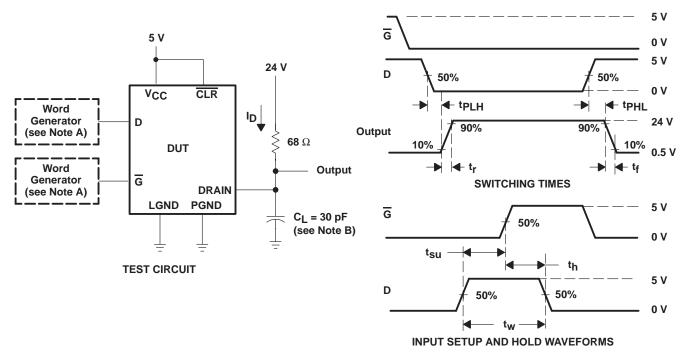
Figure 2. Test Circuit, Switching Times, and Voltage Waveforms
