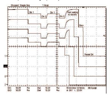
Figure 9. Four Port Discovery, Class, Power On
