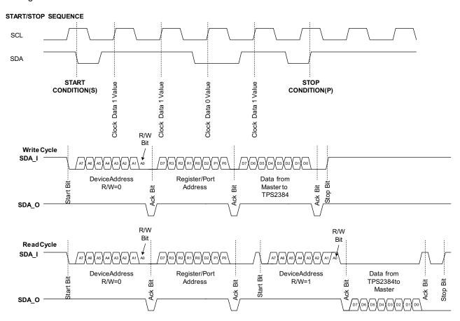
Figure 22. I<sup>2</sup>C Read/Write Cycles
