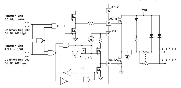
Figure 39. AC\_HI and LOW Without External FET Configurations
