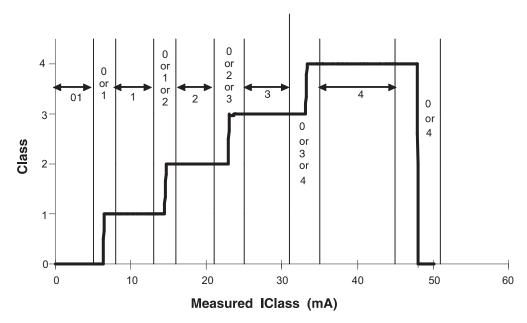
Figure 10. Class Current and Class Assignments
