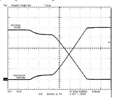
Figure 20. Rup Pwr Function Waveforms
