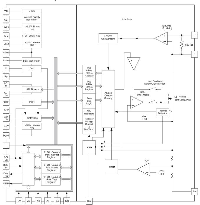
Figure 5. Single Port Block Diagram
