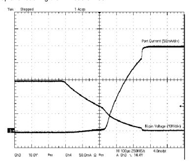
Figure 11. Port Power Delivery Voltage and Current
