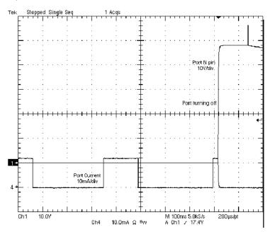
Figure 14. Port Under-current Response in DC Disconnect
