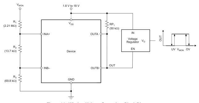
Figure 14. Window Voltage Supervisor Block Diagram
