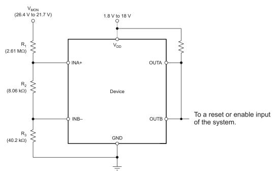
NOTE: The inputs can monitor a voltage higher than V<sub>DD</sub>max with the use of an external resistor divider network.
