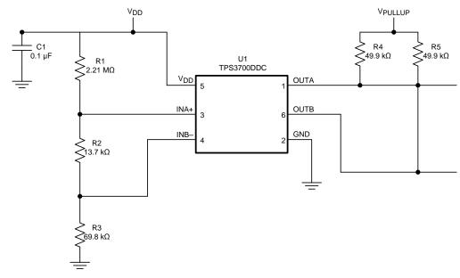
Figure 20. Typical Application Schematic
