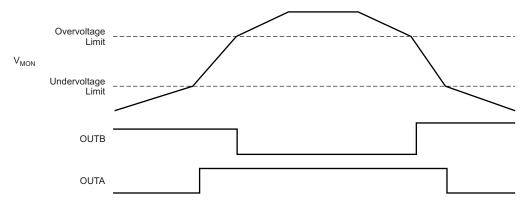
Figure 15. Window Voltage Supervisor Timing Diagram
