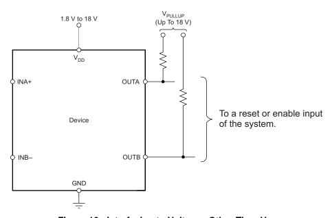
Figure 16. Interfacing to Voltages Other Than V<sub>DD</sub>
