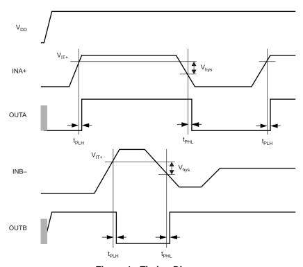
Figure 1. Timing Diagram
