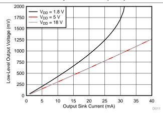
Figure 10. Output Voltage Low (V<sub>OL</sub>) vs Output Sink Current (0°C)
