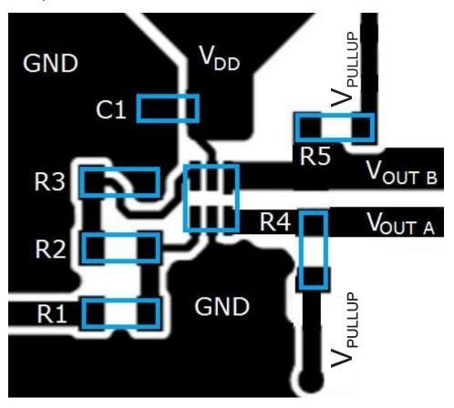
Figure 23. TPS3700 Layout Schematic
