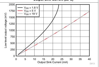
Figure 12. Output Voltage Low (V<sub>OL</sub>) vs Output Sink Current (85°C)
