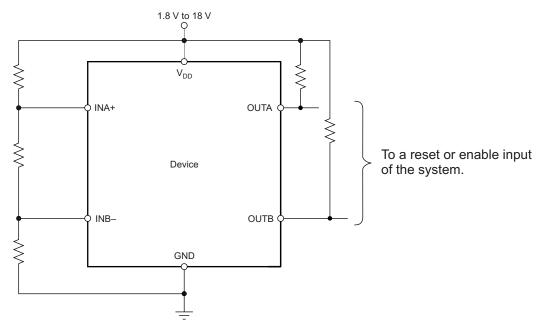
Figure 17. Monitoring the Same Voltage as V<sub>DD</sub>
