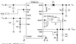
External LDO = TPS792xx series Ext. LDO nominal output voltage setting recommended at 1% lower than VMAIN.
