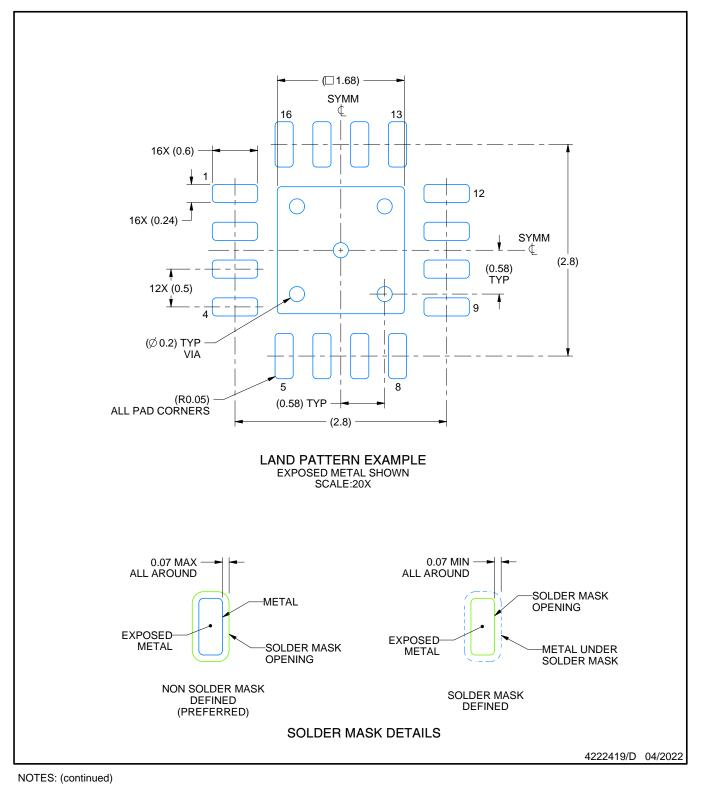
4. This package is designed to be soldered to a thermal pad on the board. For more information, see Texas Instruments literature number SLUA271 (www.ti.com/lit/slua271).
