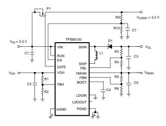
Figure 18. Power Sequencing on Digital Supply Voltage, V<sub>LOGIC</sub>
