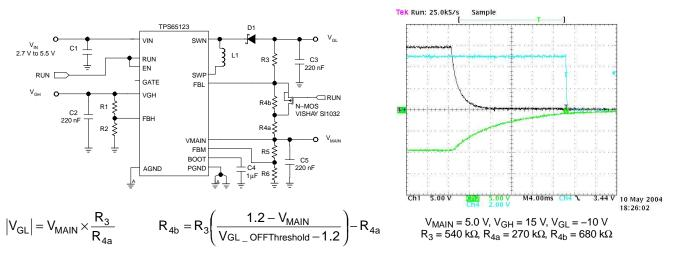
Figure 24.  $V_{GL} \rightarrow V_{MAIN}$  Power Down-Sequencing Threshold Shifting
