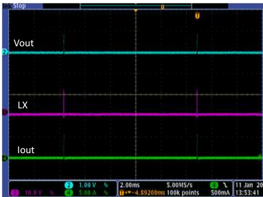
Figure 20. Buck Hiccup Response to Hard-Short Circuit
