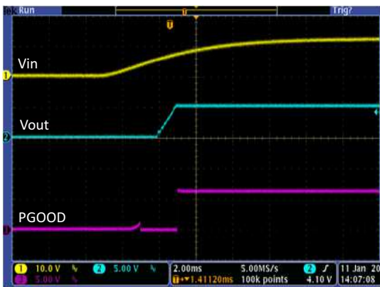
Figure 22. Power Up and PGOOD, No Load
