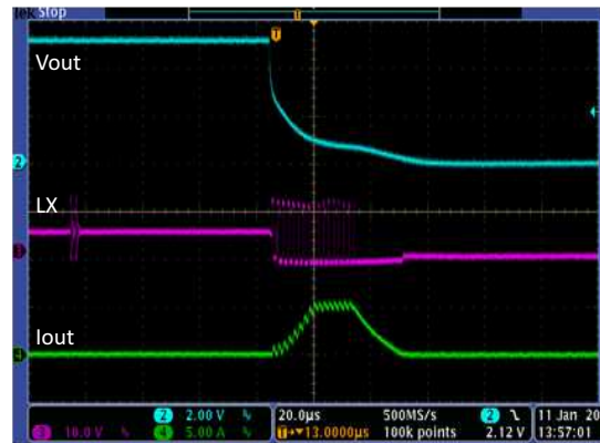
Figure 21. Zoom in Buck Output Hard-Short Response
