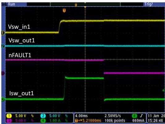
Figure 28. Power Switch1 Enable Into Short Circuit
