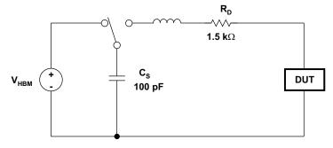
Figure 10. HBM ESD Test Circuit
