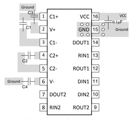
Figure 14. TRS202 Circuit Board Layout
