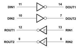
Figure 9. Logic Diagram (Positive Logic)
