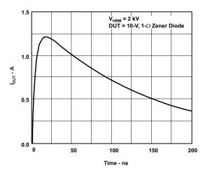
Figure 11. Typical HBM Current Waveform
