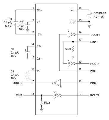
$<sup>^{\</sup>dagger}$  C3 can be connected to  $\mathrm{V}_{\mathrm{CC}}$  or GND.
