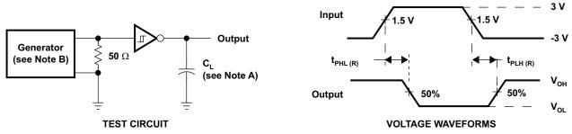
NOTES: A. C<sub>1</sub> includes probe and jig capacitance.
