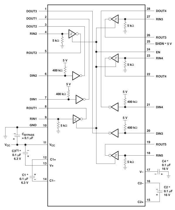
(1) C3 can be connected to  $V_{\mbox{\footnotesize CC}}$  or GND.
